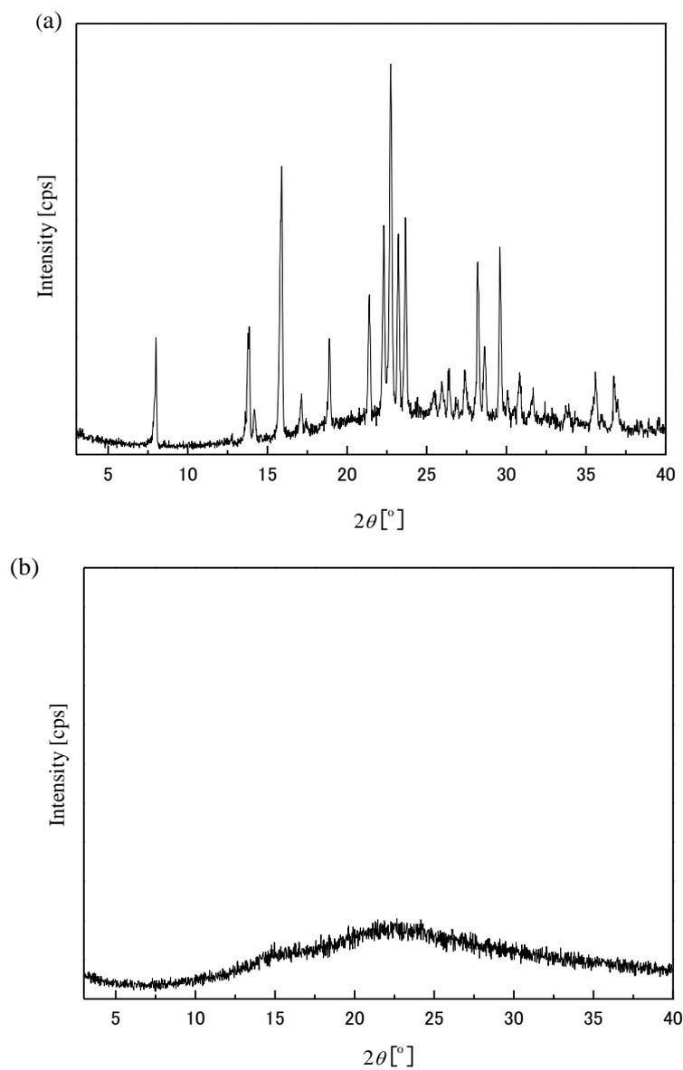
**Fig. S4.** XRD spectra of microcrystalline surface of **1o** (a) before 1<sup>st</sup> heating and (b) after second heating in Fig. S2.
