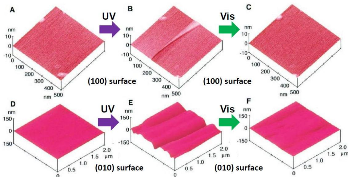
**Figure S1.** AFM images of (A to C) the (100) crystal surface of **1o** and (D to F) the (010) surface: before photoirradiation, (A) and (D); after irradiation with 366-nm light for (B) 10 s and (E) 15 s; and after irradiation with visible light ( $\lambda > 500$  nm), (C) and (F).<sup>S1</sup>
