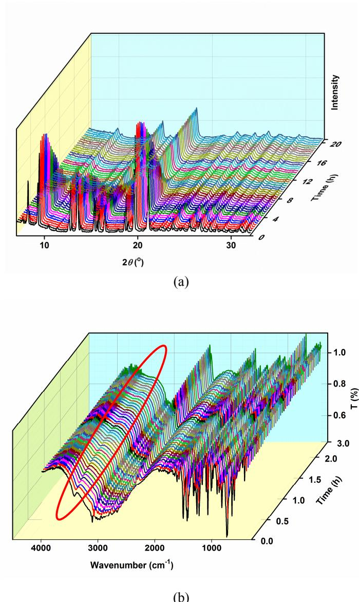
**Fig. S8** (a) Time-dependent *in situ* PXRD in dehydration process from **2**, **1** to anhydrous **L** at ambient condition. (b) Time-dependent *in situ* IR spectra in dehydration process in the flow of dried  $\text{N}_2$  at room temperature. The red circle represents the diminishing gradually of the water peaks upon the dehydration.
