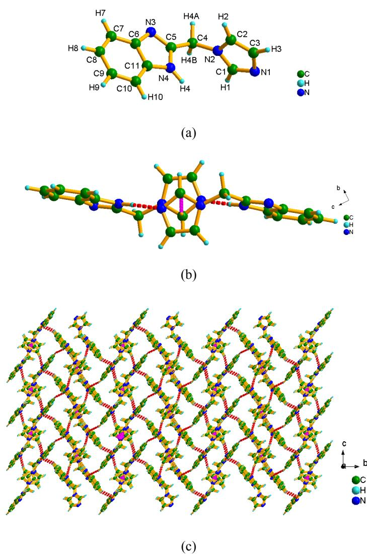
**Fig. S4** (a) Ball-stick drawing of **L** in the asymmetric unit; (b) 1D tape of **L** along the *a* axis; (c) Packing diagram in **L** along the *a* axis. The purple dashed-lines represent hydrogen bonds and stacking interactions.
