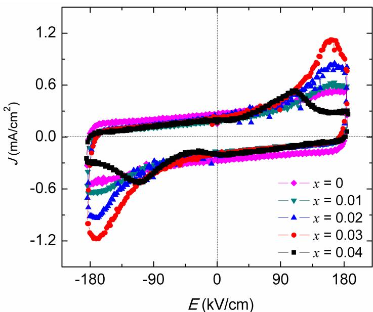
**Fig. S4** Current density hysteresis ( $J$ - $E$ ) loops of the CBNO-LiNd-ScW- $x$  ( $x = 0, 0.01, 0.02, 0.03, 0.04$ ) ceramics.
