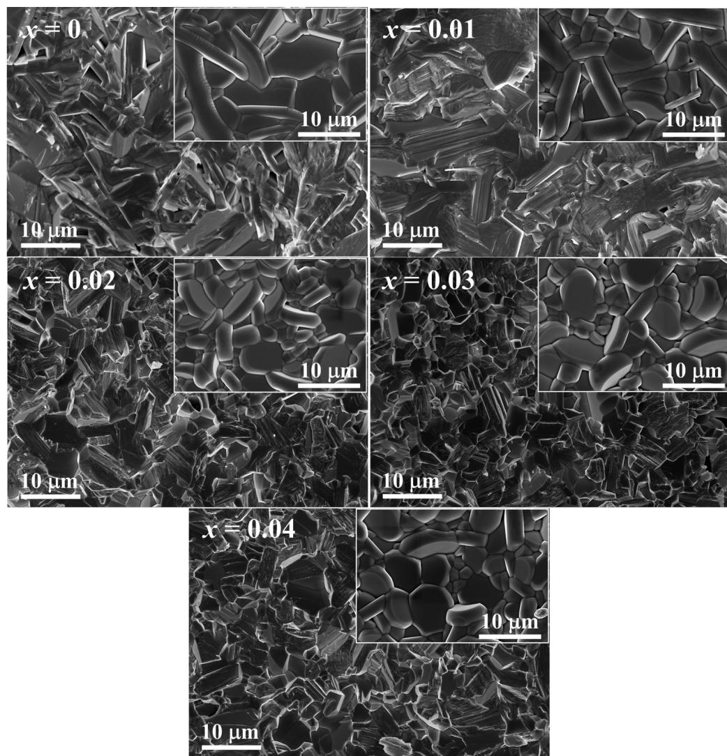
**Fig. S2** Cross-section SEM images of the prepared CBNO-LiNd-ScW- $x$  ( $x = 0, 0.01, 0.02, 0.03, 0.04$ ) ceramics, with corresponding surface morphologies as insets.
