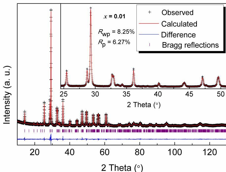
**Fig. S3** Rietveld refinement for the CBNO-LiNd-ScW-0.01 at room temperature, with an inset showing a regionally enlarged drawing.
