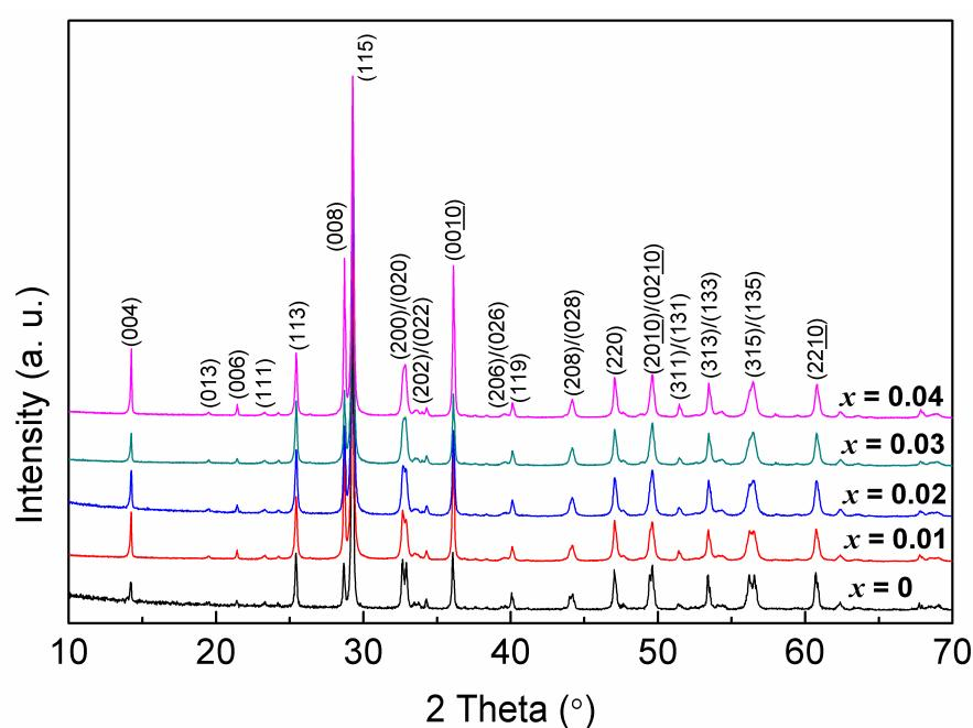
**Fig. S1** Powder XRD patterns of the CBNO-LiNd-ScW- $x$  ( $x = 0, 0.01, 0.02, 0.03, 0.04$ ) ceramics.
