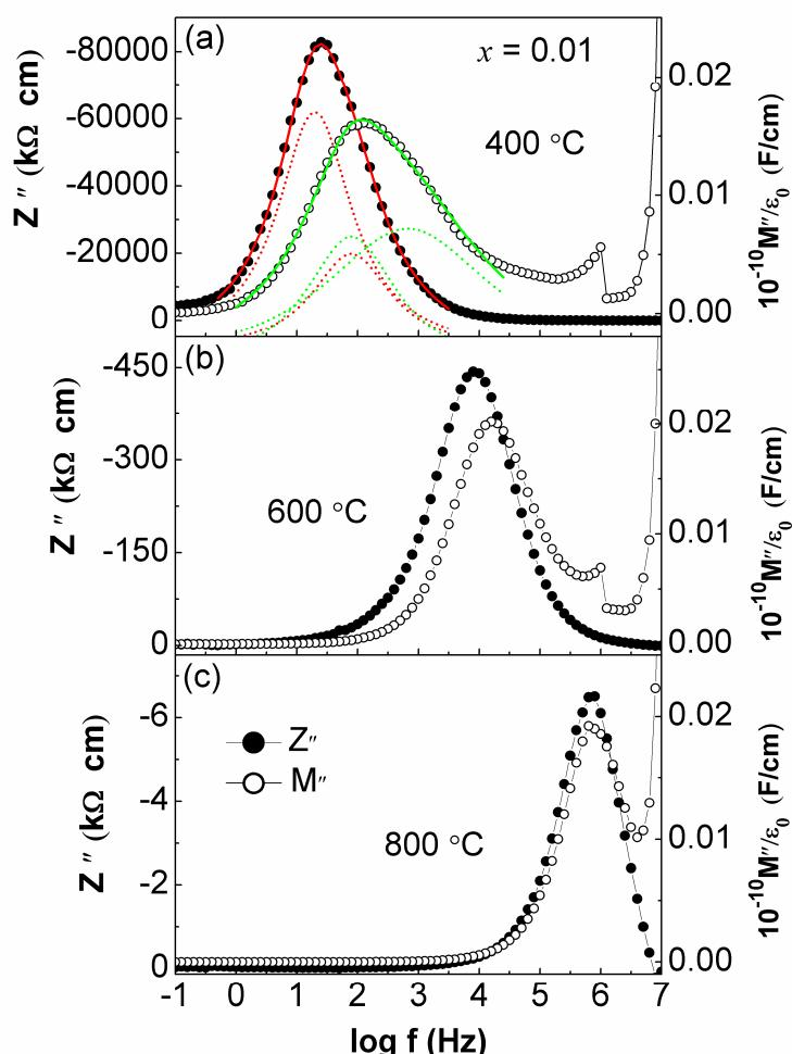
**Fig. S6** (a)  $400^\circ\text{C}$ , (b)  $600^\circ\text{C}$  and (c)  $800^\circ\text{C}$  impedance and complex modulus spectroscopic plots of the CBNO-LiNd-ScW-0.01 sample. The symbols were experimental data, the solid lines were fitting spectra, and the dotted lines were fitting peaks (the lower-frequency peak was ascribed to the effect of grain boundary while the higher-frequency peak was in response to the grain).
