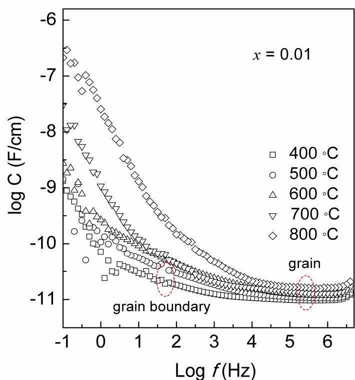
**Fig. S5** Capacitance spectroscopic plots of the CBNO-LiNd-ScW-0.01 sample with Pt electrode over 400-800 °C.
