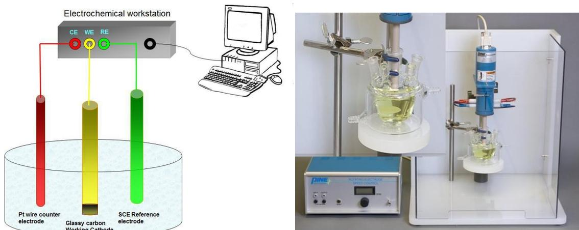
Figure S7. Schematic (left) and actual experimental (right) set-up for electrochemical measurements.
