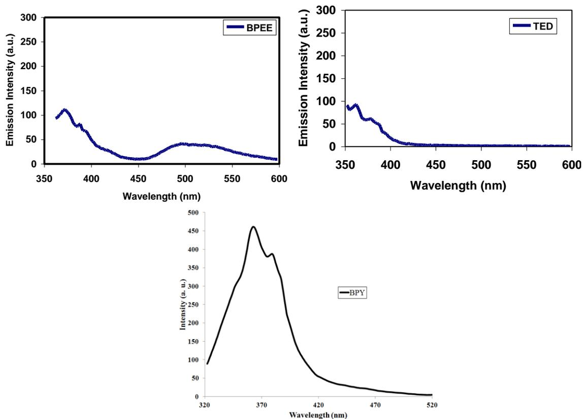
Figure S4. Emission spectra of thin-layer samples of ndc ( $\lambda_{\text{ex}}$ : 340 nm), bpe, bpee, ted ( $\lambda_{\text{ex}}$ : 330 nm) and bpy ( $\lambda_{\text{ex}}$ : 300 nm). The emission spectra of all five ligands show very little dependence on the excitation wavelength between 330 and 350 nm.
