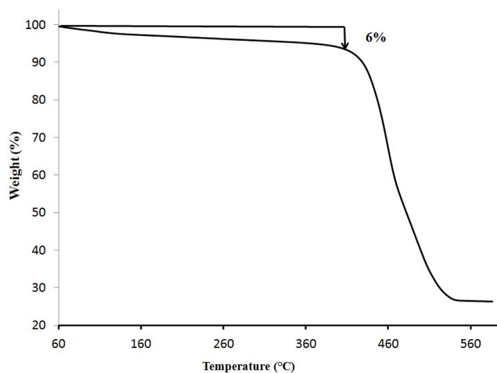
Figure S10. Observed weight loss for compound **1'** after exposure to TO vapor for 10 minutes.
