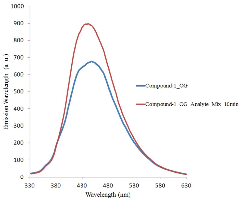
Figure S12. The effect of analytes mixture (BZ and NM (v/v) 1:1) on compound 1' (10 minutes exposure). Blue: initial PL emission spectrum of active sample 1'. Red: PL emission spectrum of 1' after 10 minutes exposure to analytes mixture at room temperature.
