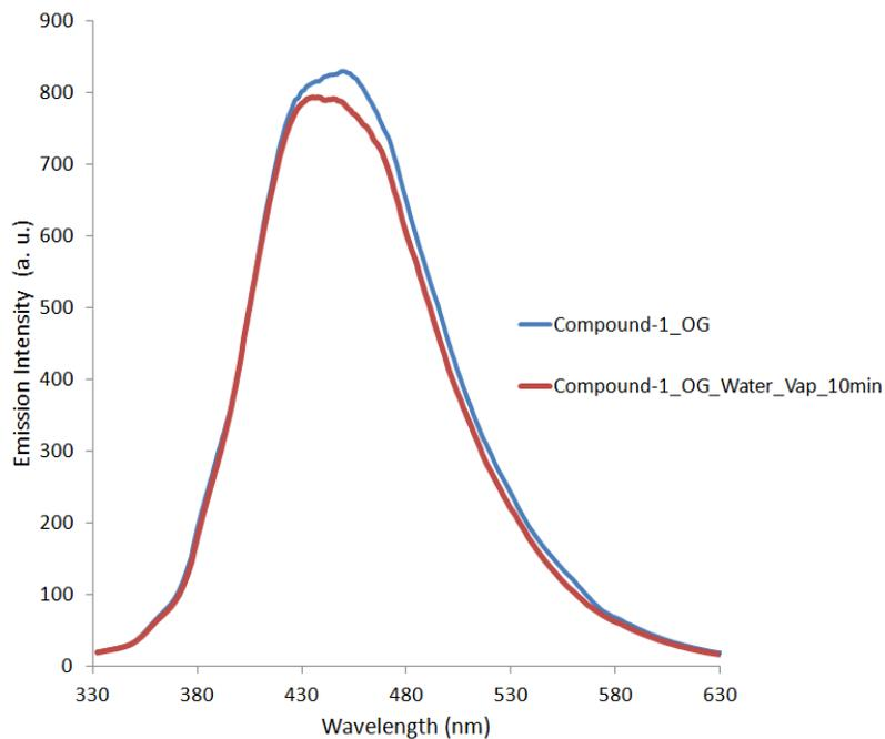
Figure S13. The effect of water vapor on the PL properties of compound **1'**. Blue: initial PL emission spectrum of activated sample **1'**. Red: PL emission spectrum of **1'** after 10 minutes exposure to air and saturated water vapor at room temperature.
