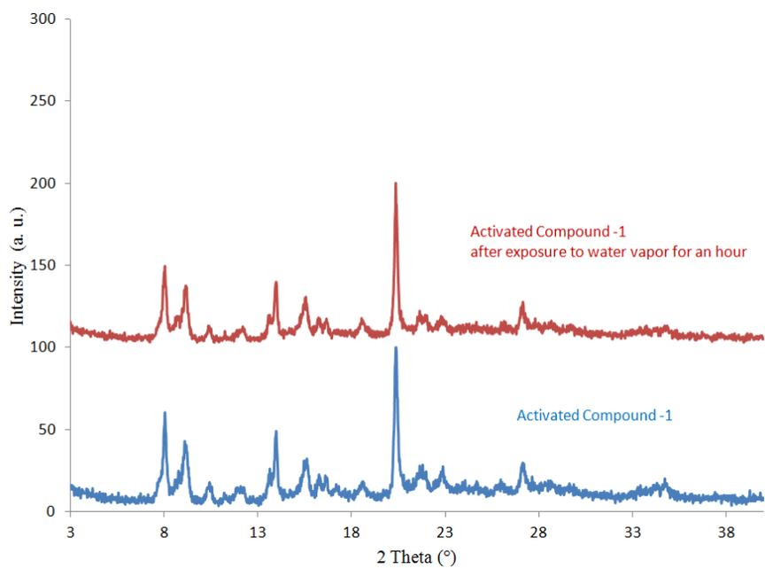
Figure S11. The stability of compound 1' in water vapor. Blue: PXRD of active sample 1'. Red: PXRD of active 1' after 1 hour exposure to saturated water vapor at room temperature.
