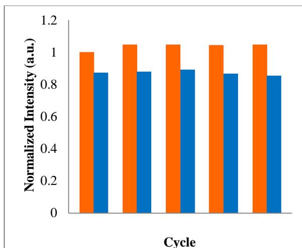
Figure S6. Recyclability test on **1'**. Nitromethane was used as a model analyte. Analyte vapor exposure time was 5 minutes. Fluorescence can be regenerated by heating the sample at 120 °C for 2 minutes. 5 consecutive cycles of quenching were achieved. Orange bar: emission of outgassed sample. Blue bar: emission after exposure to nitromethane for 5 minutes.
