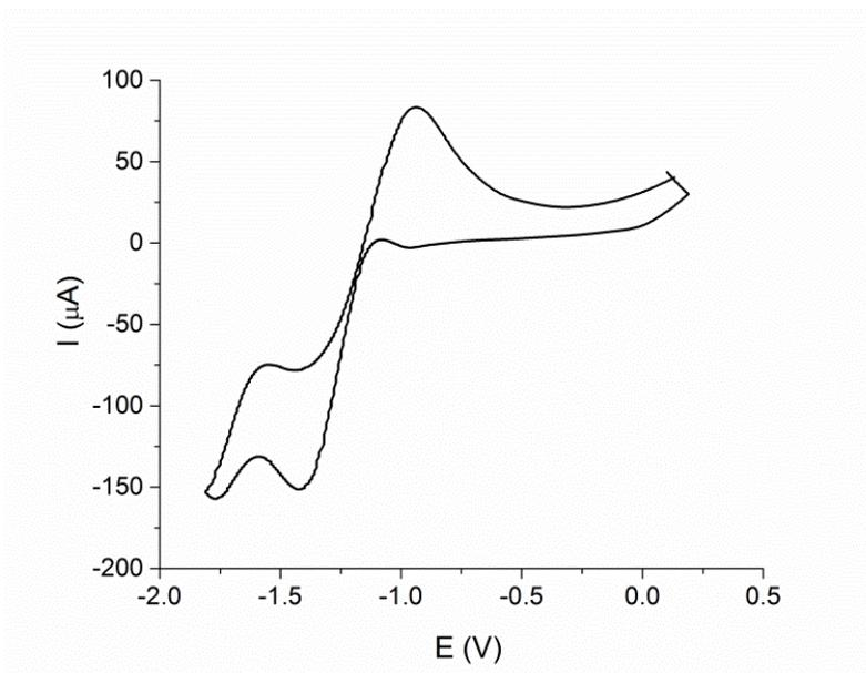
Figure S8. The CV curve of **1** measured in 0.1M LiCl in water/acetone (v/v = 3:1). The reduction potential is -1.2V after correction with the internal standard Ferrocene.
