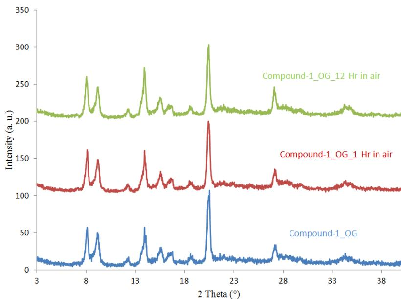
Figure S9. Stability of compound **1'** in air as observed by PXRD. Blue: PXRD pattern of activated sample **1'**. Red: PXRD pattern of **1'** after 1 hour exposure in air. Green: PXRD pattern of **1'** after 12 hours exposure in air.
