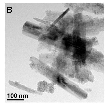
**Fig. S1** TEM images showing goethite nanorods are aggregated in samples aged at 70  $^{\circ}$ C for 4 h in the nitrate system (A), and aged at 60  $^{\circ}$ C for 5 h in the sulfate system (B). Average particle size by XRD analyses is 33 nm for (A) and 36 nm for (B).
