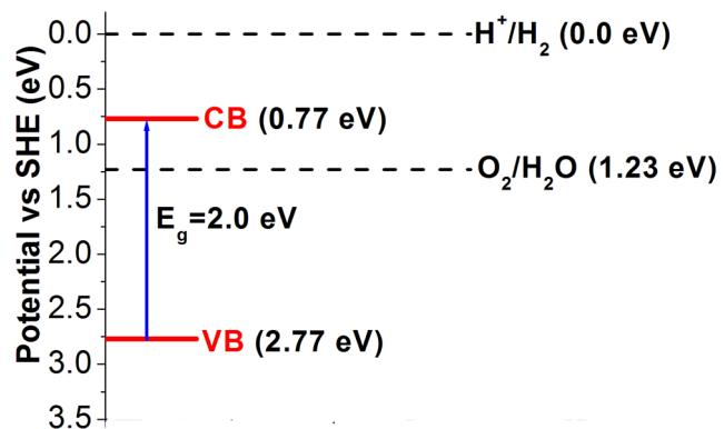
Fig. S6. Schematic band structure of FeVO<sub>4</sub>-II.
