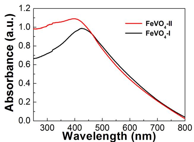
Fig. S4. UV-Vis diffuse reflectance spectroscopy of  $\text{FeVO}_4\text{-II}$  and  $\text{FeVO}_4\text{-I}$  photocatalysts.
