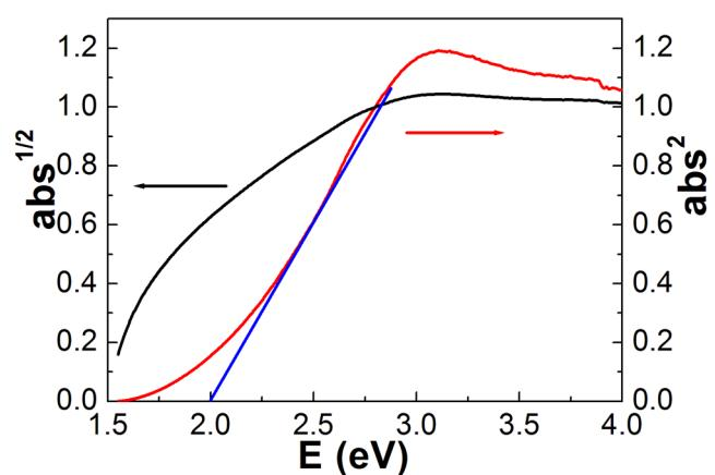
Fig. S5. The plots of absorption squared ( $\text{abs}^2$ ) and the square root of absorption ( $\text{abs}^{1/2}$ ) versus energy for the  $\text{FeVO}_4\text{-II}$  absorption in the absorption edge region of  $\text{FeVO}_4\text{-II}$  sample.
