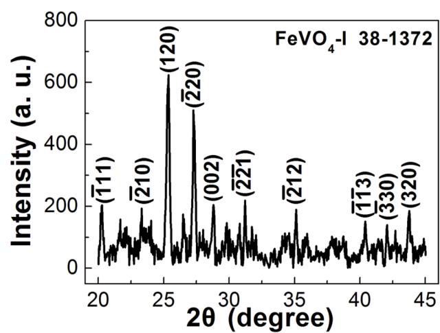
Fig. S1. (a) XRD pattern of the as-prepared products showing triclinic phase of FeVO<sub>4</sub>-I.
