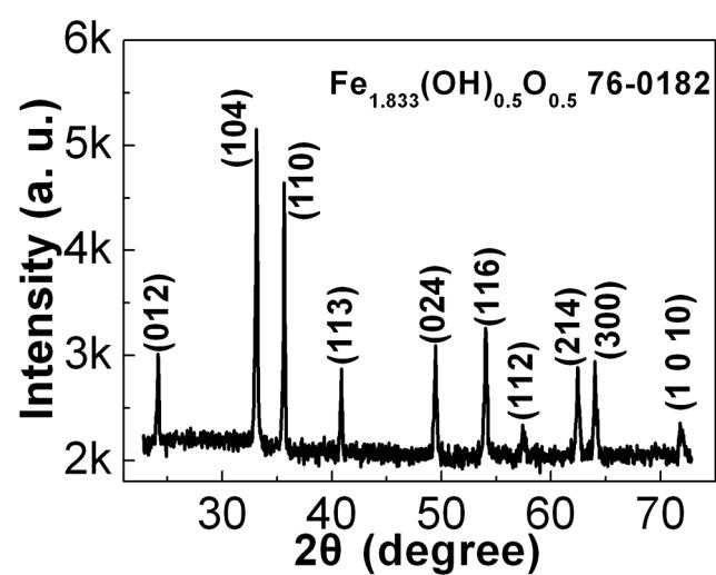
Fig. S3. XRD pattern of the products showing hexagonal  $\text{Fe}_{1.833}(\text{OH})_{0.5}\text{O}_{0.5}$  at pH 12.
