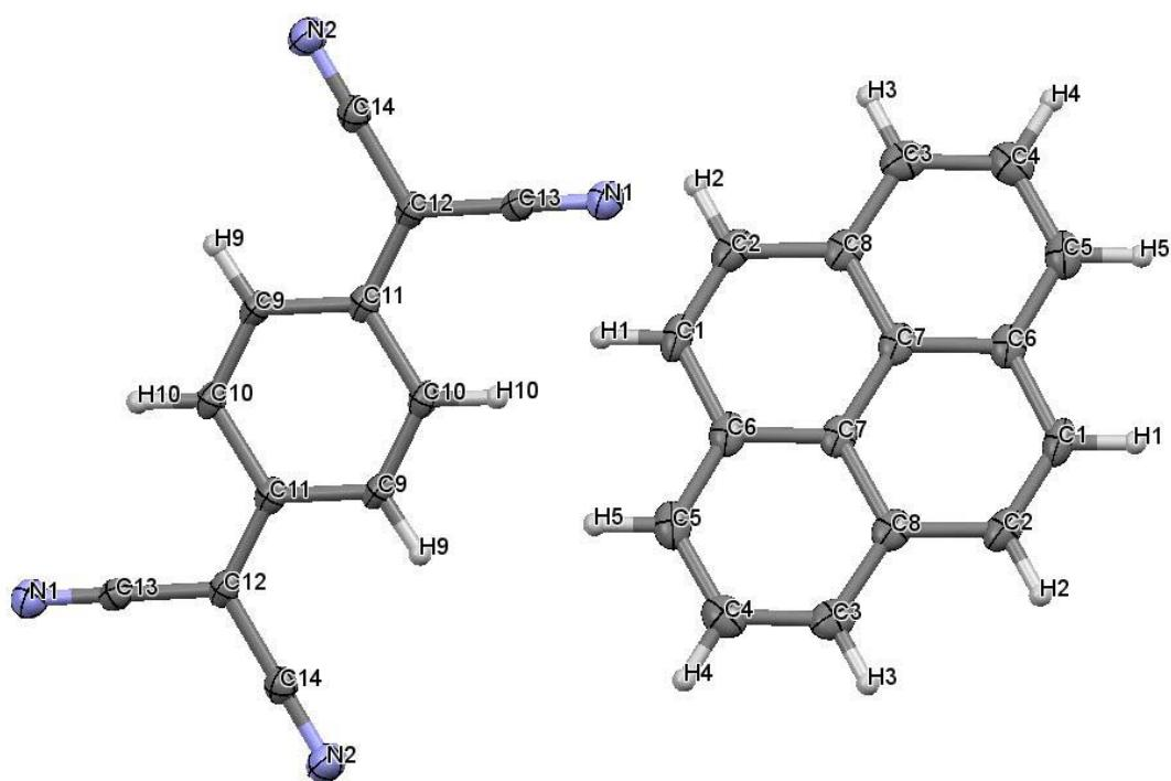
Fig. S4. The molecular structure of (**4**) showing displacement ellipsoid at the 50% probability level.
