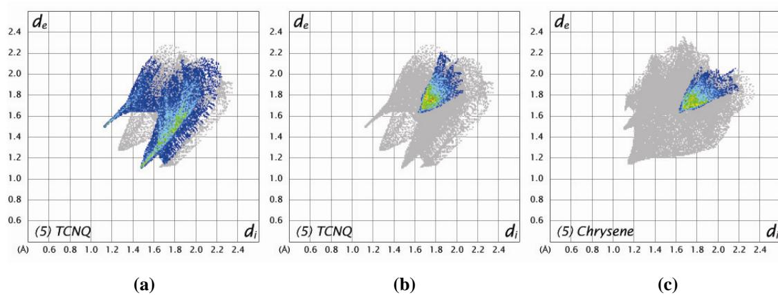
Fig. S11. Fingerprint plots visualizing  $d_e$  and  $d_i$  for N···H (a) and C···C contacts (b), (c) (including reciprocal ones) generated for TCNQ and chrysene molecules in complex (5).
