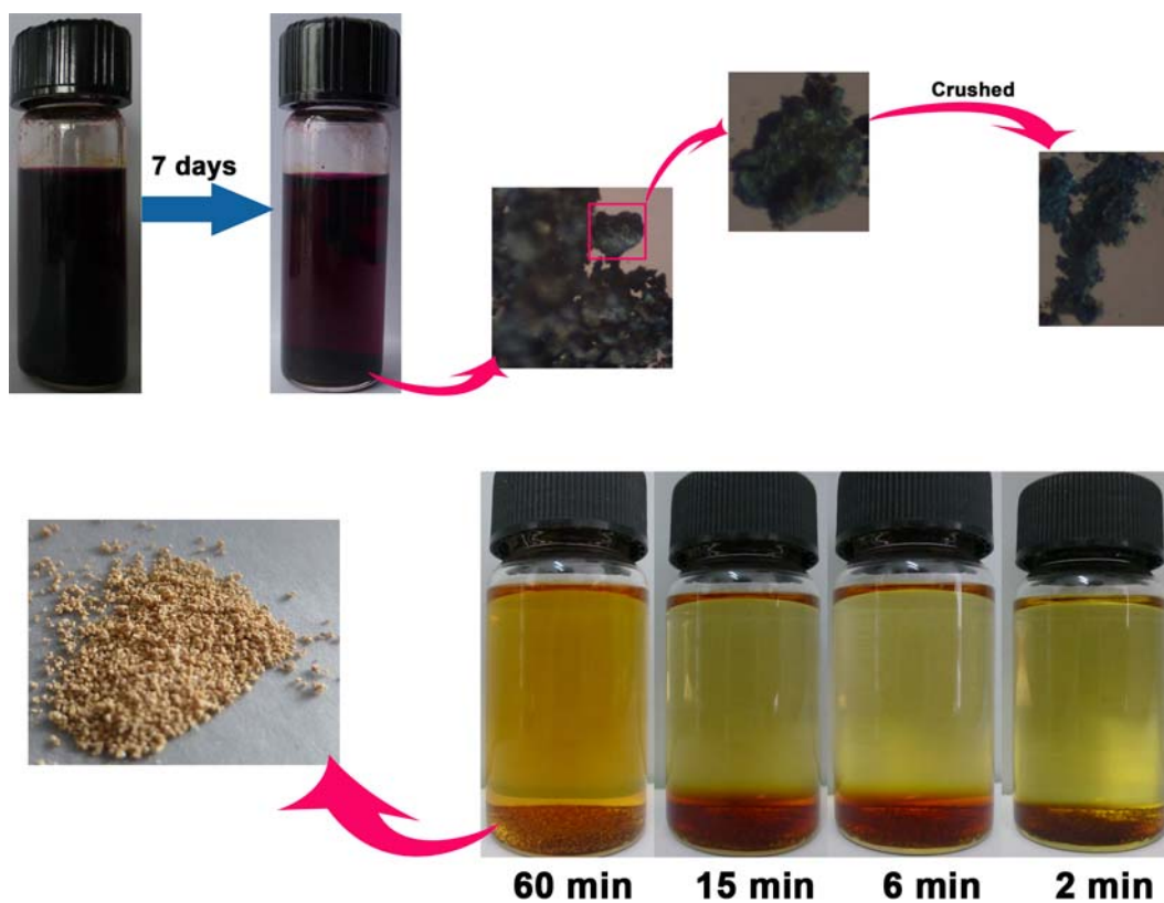
Fig. S8 Up: Photos of the iodine recovery process with 100 mg of 1 soaked in cyclohexane solution of I 2 (0.1 M/L, 3 mL). Down: I 2 releasing process of 1 \supset I 2 (30 mg in 20 mL of EtOH).
