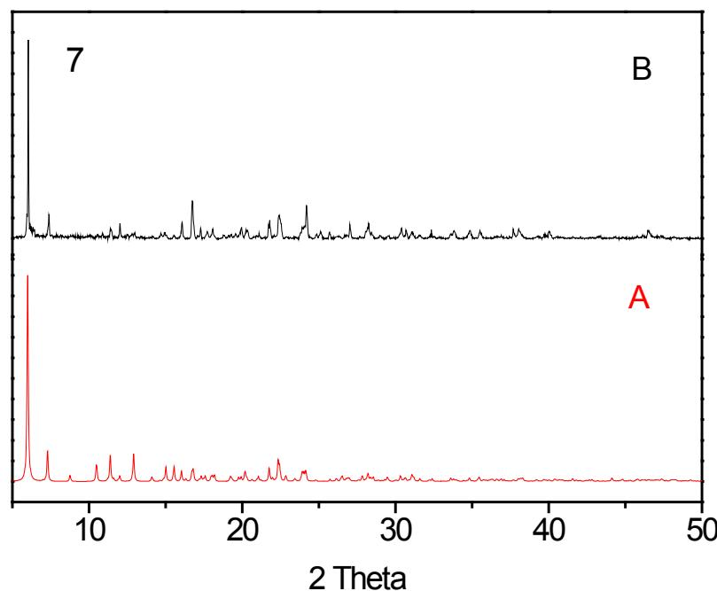
**Fig. S8** Simulated A (red) and measured B (black) PXRD patterns of **1–7**.
