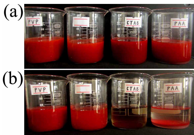
Fig. S7. (a) The instantaneous digital image of adding different surfactants. (b) The digital image of adding different surfactants after 3 hours at room temperature. The second beakers are the reaction reagents with no surfactant.
