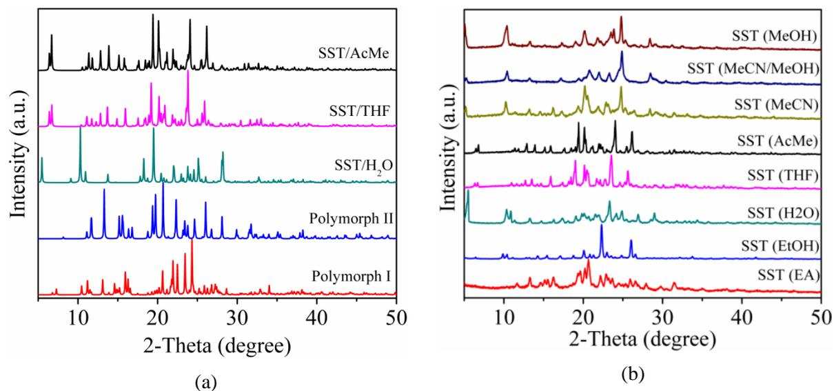
**Figure S3.** PXRD of (a) simulated and (b) experimental patterns of FE product, of succinylsulfathiazole polymorphs, hydrate and solvates (THF and AcMe).
