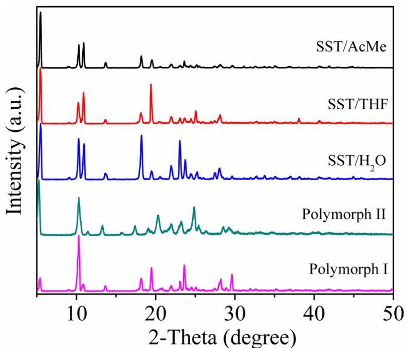
**Figure S4.** PXRD patterns of different forms of SST after a long exposure (1 yr) to atmosphere confirm their conversion to SST·H<sub>2</sub>O, except polymorph II which is converted to SST·2H<sub>2</sub>O (Fig. S2a).
