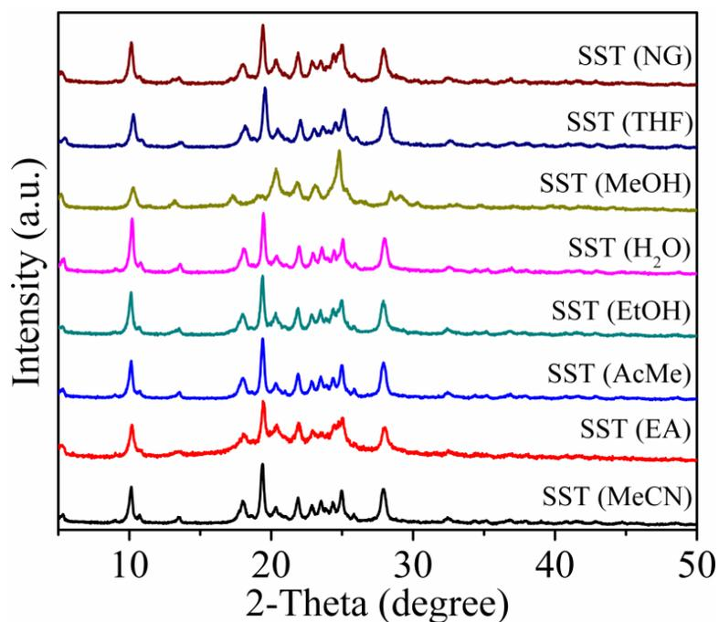
**Figure S5.** PXRD pattern of SST obtained by LAG method from different solvents. Notice the similarity of patterns of all the LAG products, which correspond to SST·H<sub>2</sub>O.
