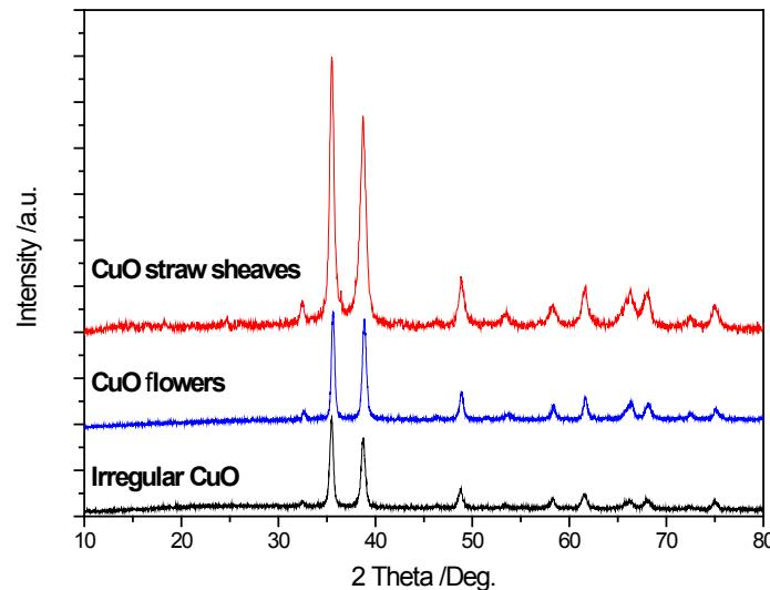
**Fig. S7** XRD patterns of the CuO samples
