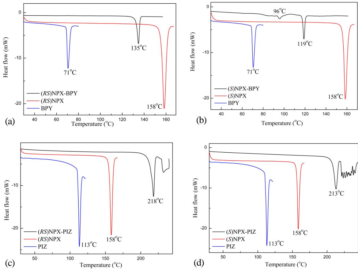
**Fig. SF3** DSC plots of naproxen cocrystals and their components (a) RS-NPX-BPY, (b) S-NPX-BPY, (c) RS-NPX-PIZ and (d) S-NPX-PIZ.
