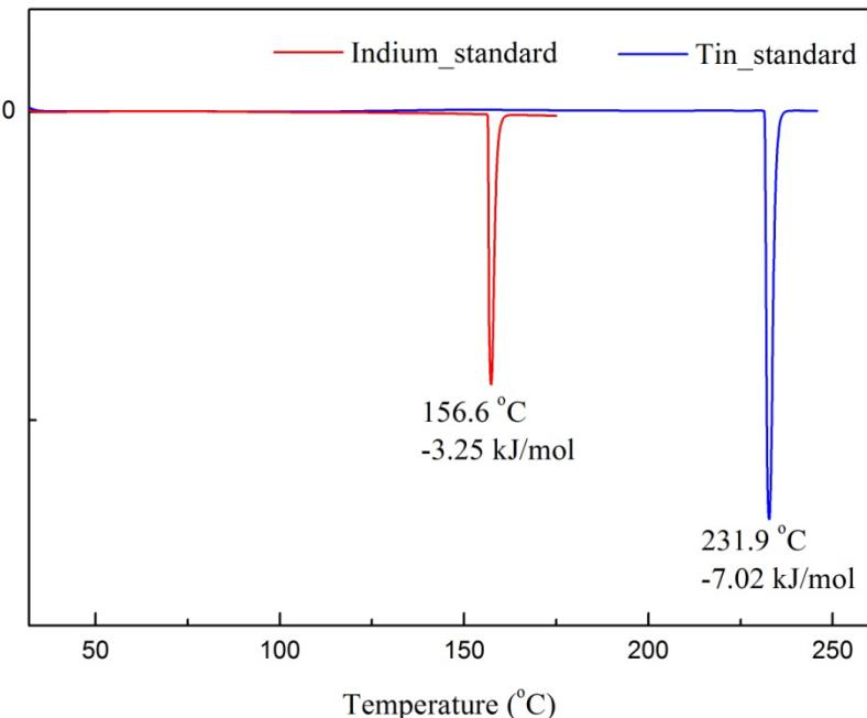
**Fig. SF4** DSC plots of Indium and Tin standard for showing the calibration of DSC instrument.
