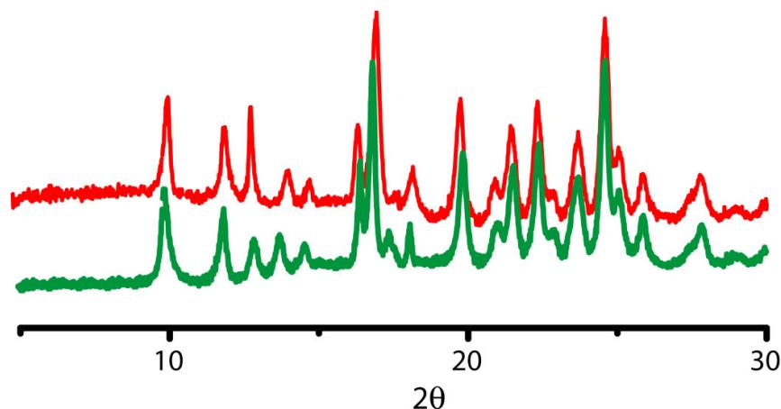
**Fig. S23.** PXRD pattern of water adsorbed sample of compound **3**; As-synthesized (green), H<sub>2</sub>O adsorbed (red).
