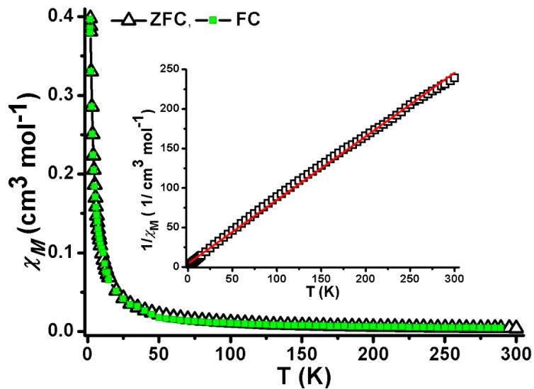
**Fig. S14.** Temperature dependence of the FC and ZFC susceptibility ( $\chi_M$ ) of **2** at 0.01 T. Inset shows temperature dependence of  $1/\chi_M$ . The red solid line represents the Curie-Weiss fitting to the curve.
