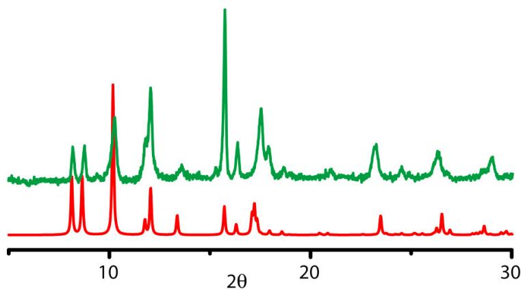
**Fig. S10.** PXRD patterns of compound **1**; Simulated (red), As-synthesized (green).
