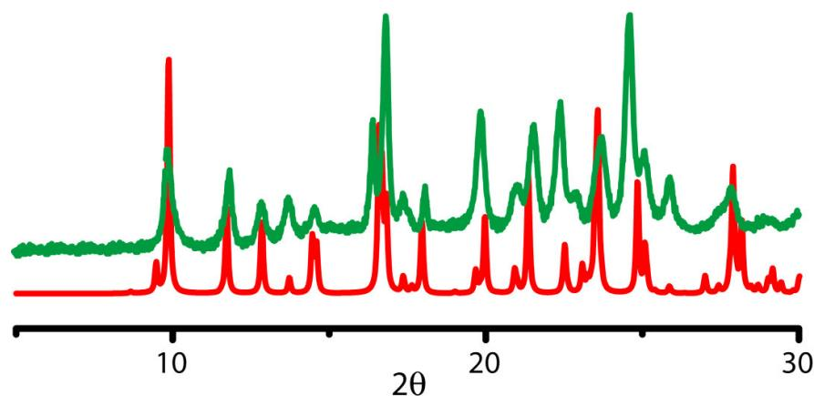
**Fig. S12.** PXRD patterns of compound **3**; Simulated (red), As-synthesized (green).
