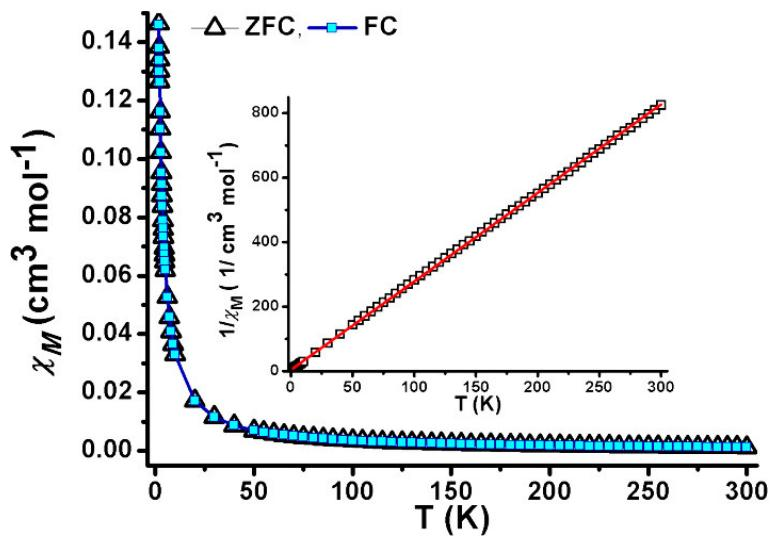
**Fig. S16.** Temperature dependence of the FC and ZFC susceptibility ( $\chi_M$ ) of **3** at 0.01 T. Inset shows temperature dependence of  $1/\chi_M$ . The red solid line represents the Curie-Weiss fitting to the curve.
