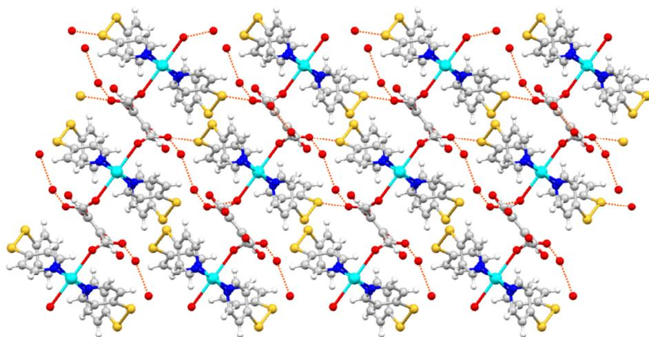
**Fig. S8.** Illustration of 3D networks found in 3 through H-bonding interaction between 2D layers through solvated water molecules. Colour code. Copper(cyan), Oxygen(red), Nitrogen(blue), Carbon(light grey), Sulphur(yellow).
