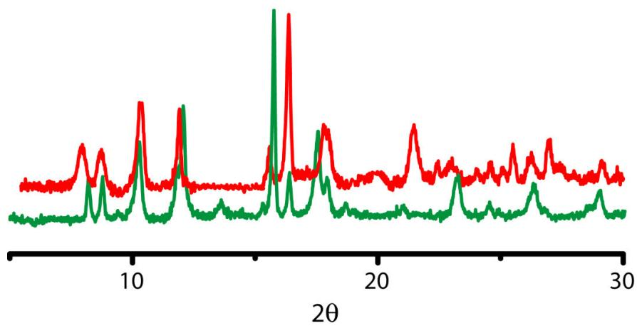
**Fig. S21.** PXRD pattern of water adsorbed sample of compound **1**; As-synthesized (green), H<sub>2</sub>O adsorbed (red).
