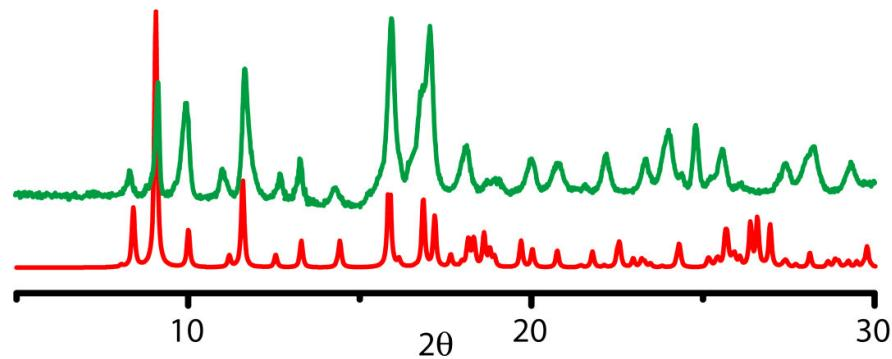
**Fig. S11.** PXRD patterns of compound **2**; Simulated (red), As-synthesized (green).
