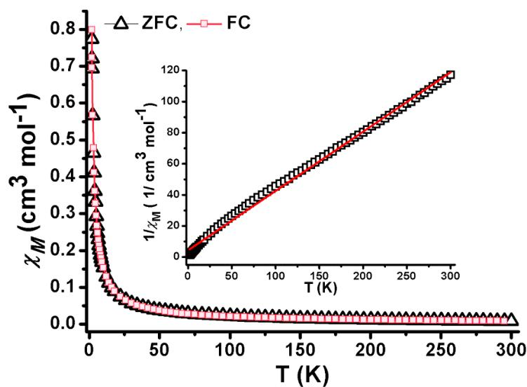
**Fig. S13.** Temperature dependence of the FC and ZFC susceptibility ( $\chi_M$ ) of **1** at 0.1 T. Inset shows temperature dependence of  $1/\chi_M$ . The red solid line represents the Curie-Weiss fitting to the curve.
