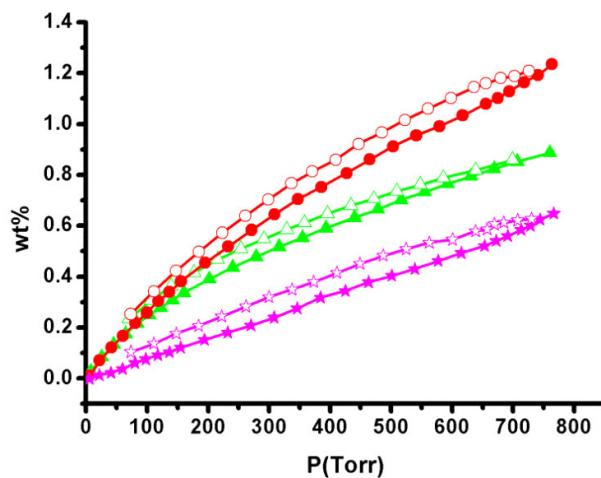
**Fig. S19.** CO<sub>2</sub> adsorption isotherms of compounds **1-3** at 298 K. **1**(magenta), **2**(green), **3**(red).
