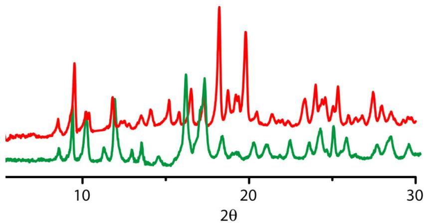
**Fig. S22.** PXRD pattern of water adsorbed sample of compound **2**; As-synthesized (green), H<sub>2</sub>O adsorbed (red).
