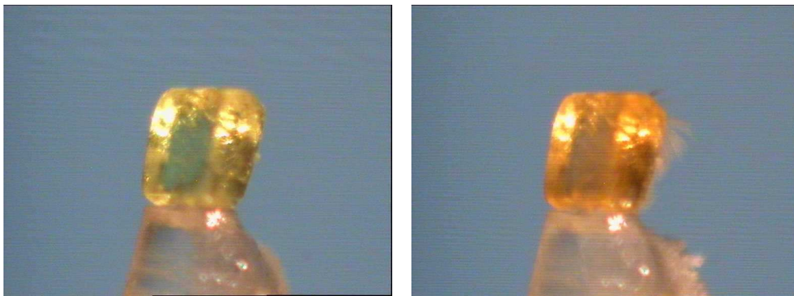
Figure S53. Photographs showing solid-state thermochromism of 6 at a) 298 and b) 110 K.
