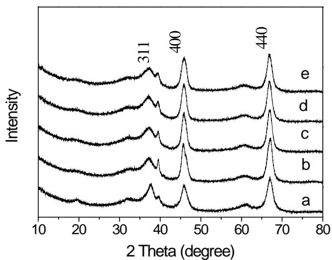
**Fig. S4.** XRD patterns of the calcined samples a)  $\eta$ - $\text{Al}_2\text{O}_3$  calcined by bayerite precursor, b)  $\text{Al}_2\text{O}_3$ -0HAc, c)  $\text{Al}_2\text{O}_3$ -10HAc, d)  $\text{Al}_2\text{O}_3$ -20HAc and e)  $\text{Al}_2\text{O}_3$ -40HAc.
