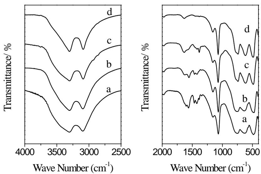
**Fig. S3.** FT-IR spectra of the obtained samples Al-HAc (a and b) and Al-NH<sub>4</sub>Ac (c and d) before (a and c) and after (b and d) washing.
