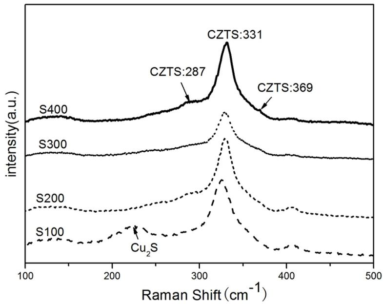
**Figure. S2** Raman spectra of the CZTS nanocrystalline thin films samples prepared for 18 h at 250 °C on stainless steel substrates. The thicknesses of CuSnZn alloy layers are 100 nm~400 nm.
