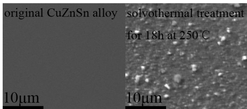
Figure S8 SEM images of the original and solvothermal treated alloy surface.
