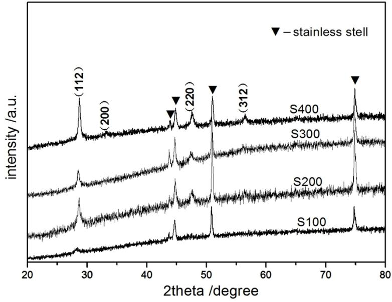
**Figure. S1** XRD patterns of the CZTS nanocrystalline thin films samples prepared for 18 h at 250 °C on stainless steel substrates. The thicknesses of CuSnZn alloy layers were 100 nm~400 nm.
