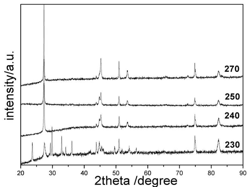
**Figure. S3** XRD patterns of the CZTSe nanocrystalline thin films samples prepared at 230~270 °C for 18 h on stainless steel substrates. The thickness of CuSnZn alloy layer is 400 nm.
