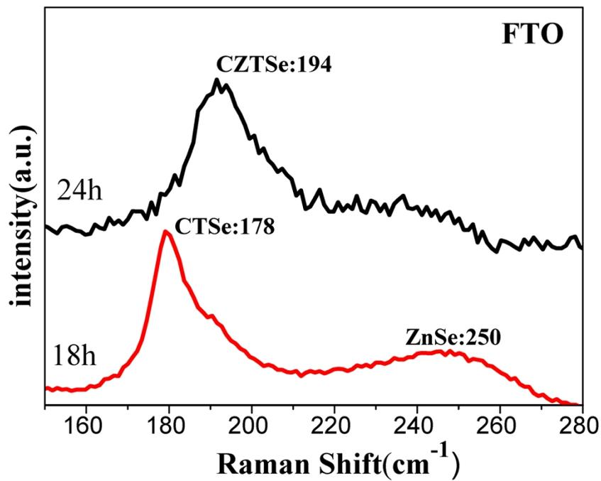
**Figure. S5** Raman spectra of the CZTSe nanocrystalline thin films samples prepared for 18 h and 24 h at 250 °C on FTO substrates.
