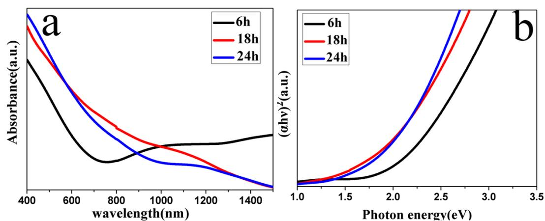
Figure S7 UV-vis-NIR absorption spectra of the CZTS thin film prepared at 250°C for 6 h, 18 h and 24 h (a) and the corresponding  $(\alpha h\nu)^2$  vs.  $h\nu$  curves (b).
