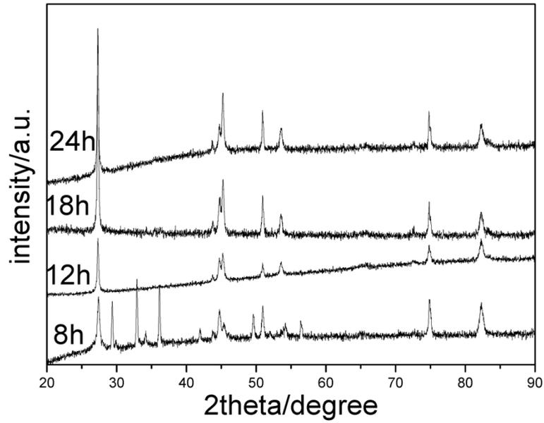
**Figure. S4** XRD patterns of the CZTSe nanocrystalline thin films samples prepared for 18h~24h at 250 °C on stainless steel substrates. The thickness of CuSnZn alloy layer is 400nm.
