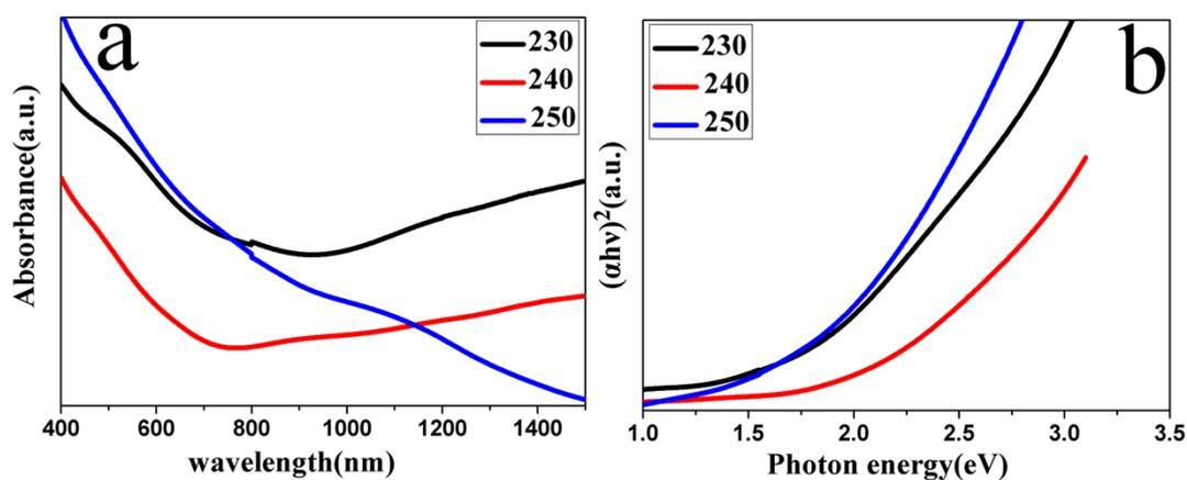
Figure S6 UV-vis-NIR absorption spectra of the CZTS thin film prepared at 230°C, 240°C and 250°C for 18 h (a) and the corresponding  $(\alpha h\nu)^2$  vs.  $h\nu$  curve (b).
