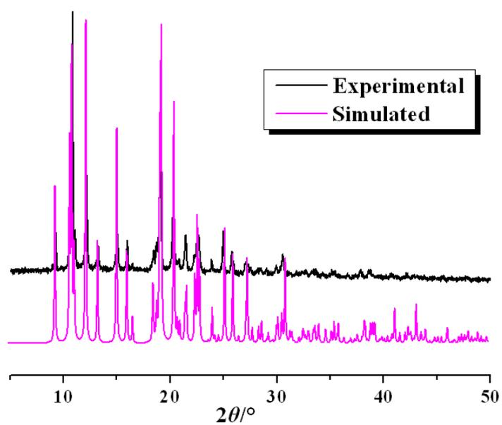
**Fig. S6** The simulated (purple) and the experimental (black) PXRD patterns of **4**.
