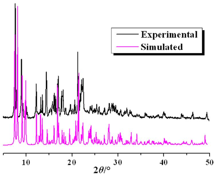
**Fig. S4** The simulated (purple) and the experimental (black) PXRD patterns of **2**.
