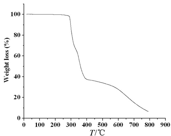
**Fig. S9** TG curve from room temperature to 800 °C for **1**.
