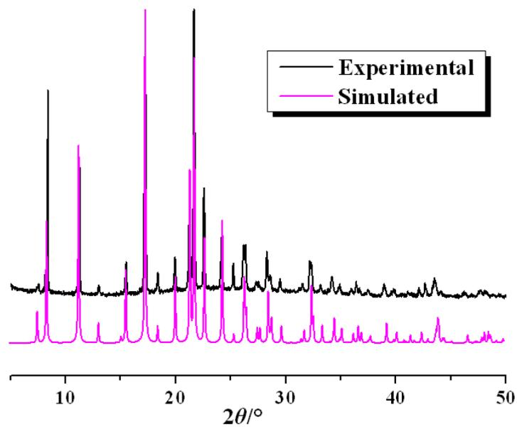
**Fig. S3** The simulated (purple) and the experimental (black) PXRD patterns of **1**.
