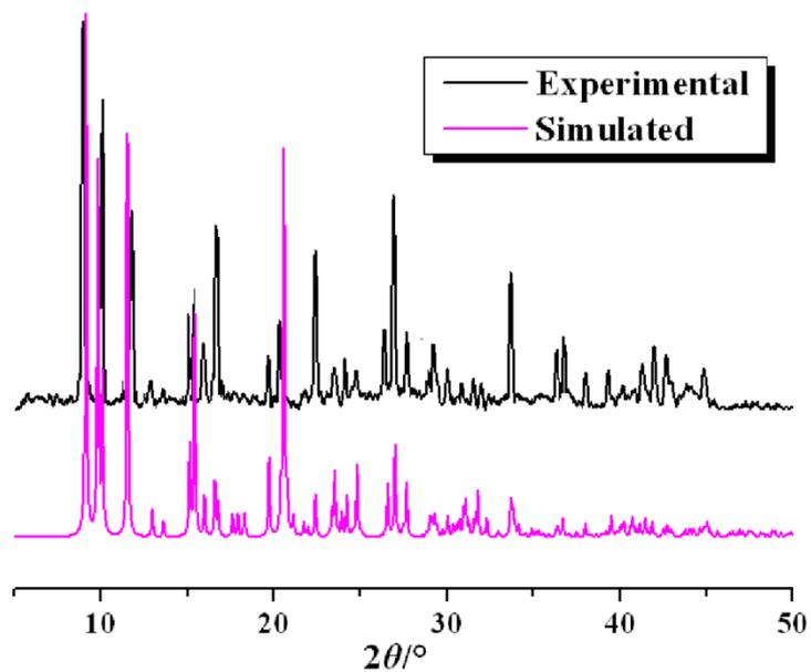
**Fig. S5** The simulated (purple) and the experimental (black) PXRD patterns of **3**.
