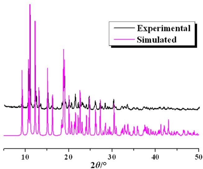
**Fig. S7** The simulated (purple) and the experimental (black) PXRD patterns of **5**.
