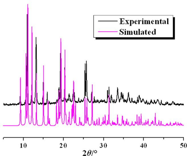
**Fig. S8** The simulated (purple) and the experimental (black) PXRD patterns of **6**.
