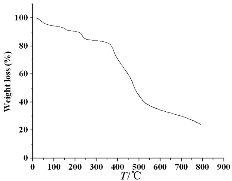
**Fig. S10** TG curve from room temperature to 800 °C for **2**.
