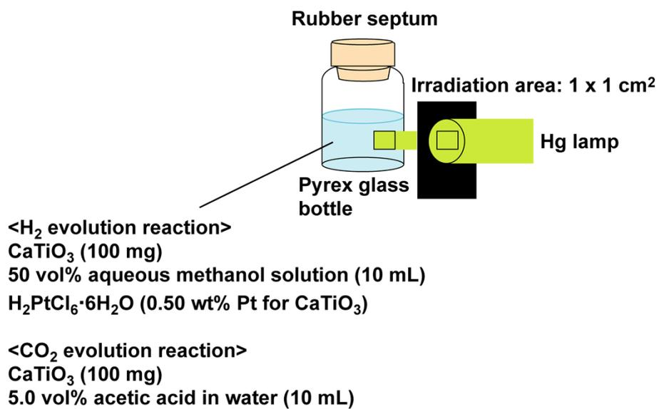
**Figure S1.** Schematic illustration for H<sub>2</sub> and CO<sub>2</sub> evolution reaction.
