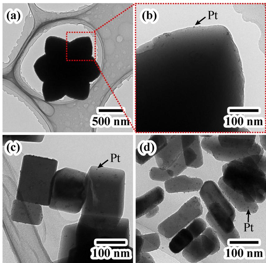
**Figure S5.** TEM images of Pt-loaded (a, b) concave cubic-, (c) cubic-, and (d) rod-shaped particles after  $H_2$  evolution reaction.
