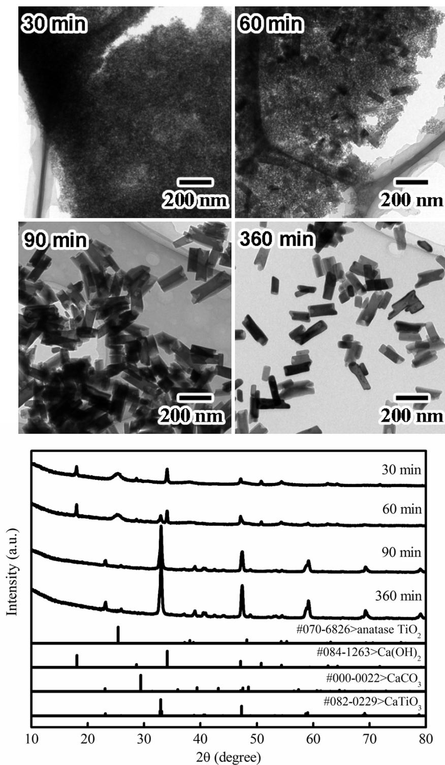
**Figure S2.** TEM images and XRD patterns of particles obtained at the same condition as CT4 except for aging time. The aging time was varied from 30 to 360 min.
