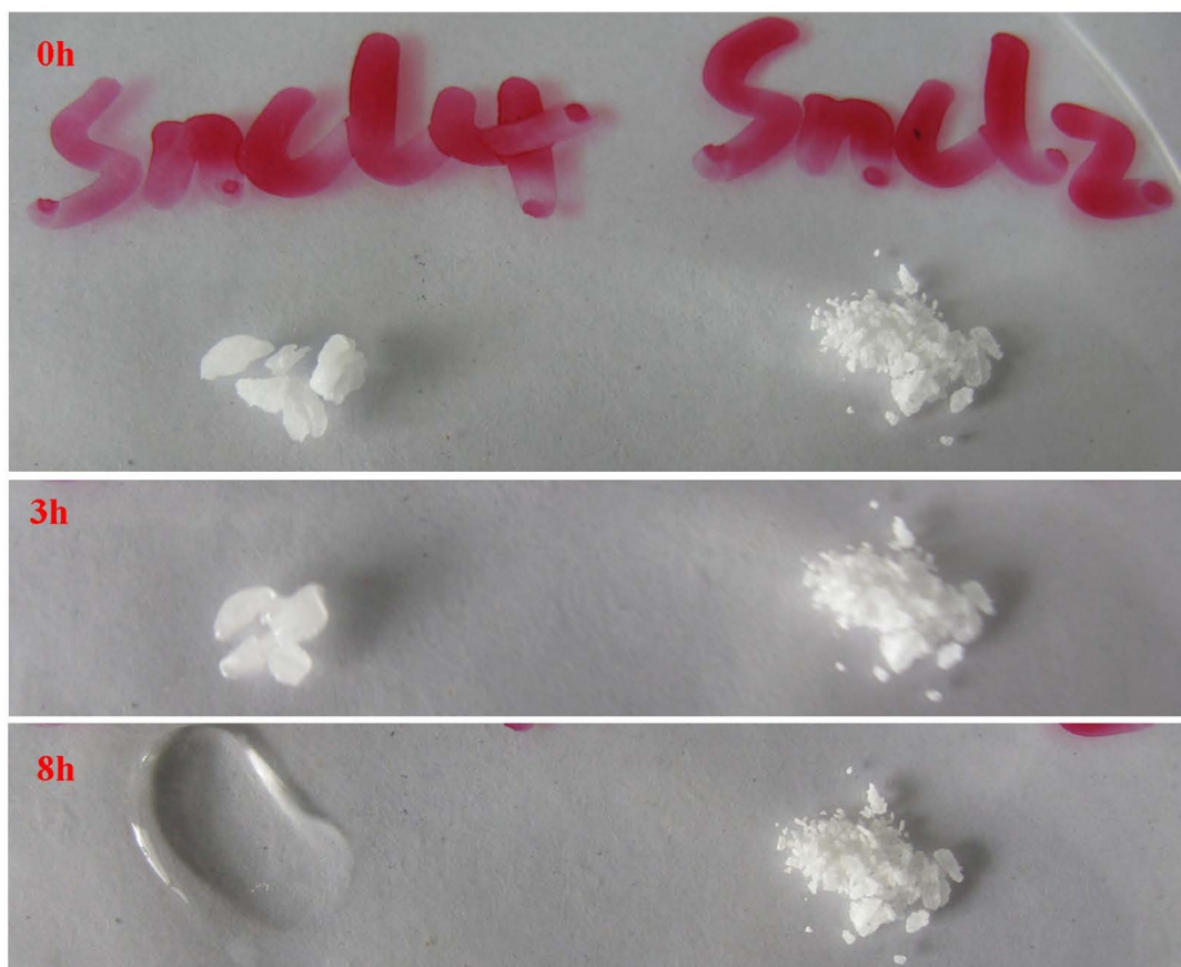
Figure S3. Photograph of the change of \text{SnCl}_4 and \text{SnCl}_2 salts in air after different aging time.
