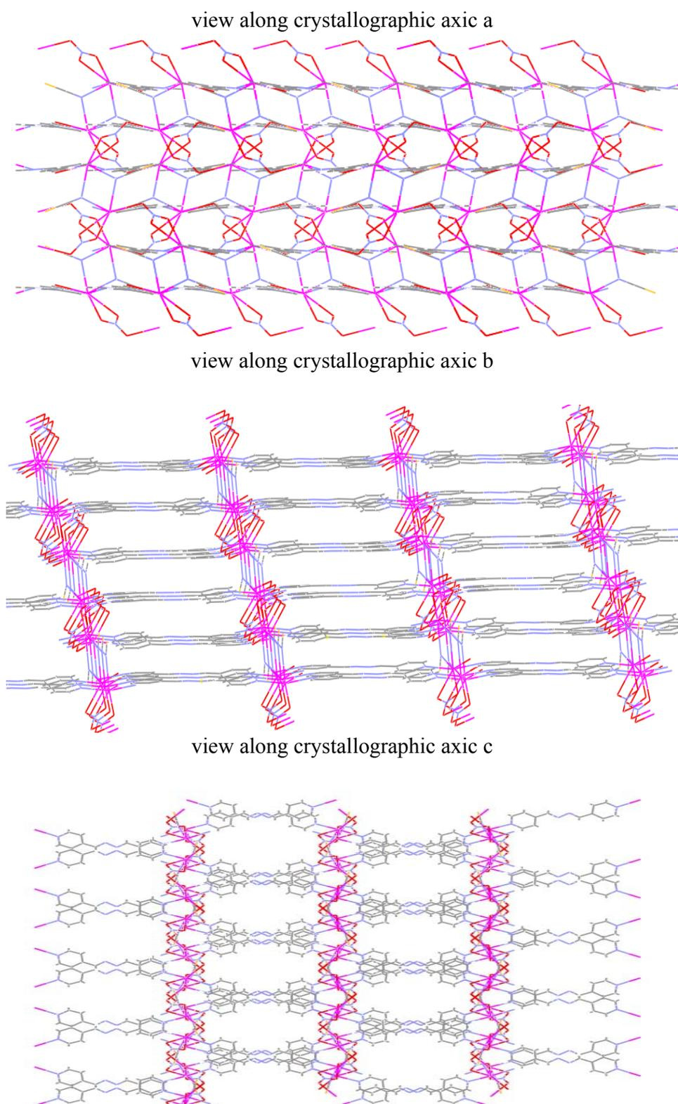
**Fig. S3.** A fragment of nano-porous 3D coordination polymer in  $[\text{Pb}(4\text{-bpdb})(\mu\text{-NO}_3)(\mu\text{-SCN})]_n \cdot 1.5 \text{CH}_3\text{OH}$  (**TMU-15**) (view along crystallographic axis a, b and c). The lead atoms are connected into infinite chains through the  $(\text{C}_{10}\text{H}_{10}\text{N}_4)$  ligands and the chains are further linked into MOF by  $\text{NO}_3^-$  and  $\text{SCN}^-$  anions.
