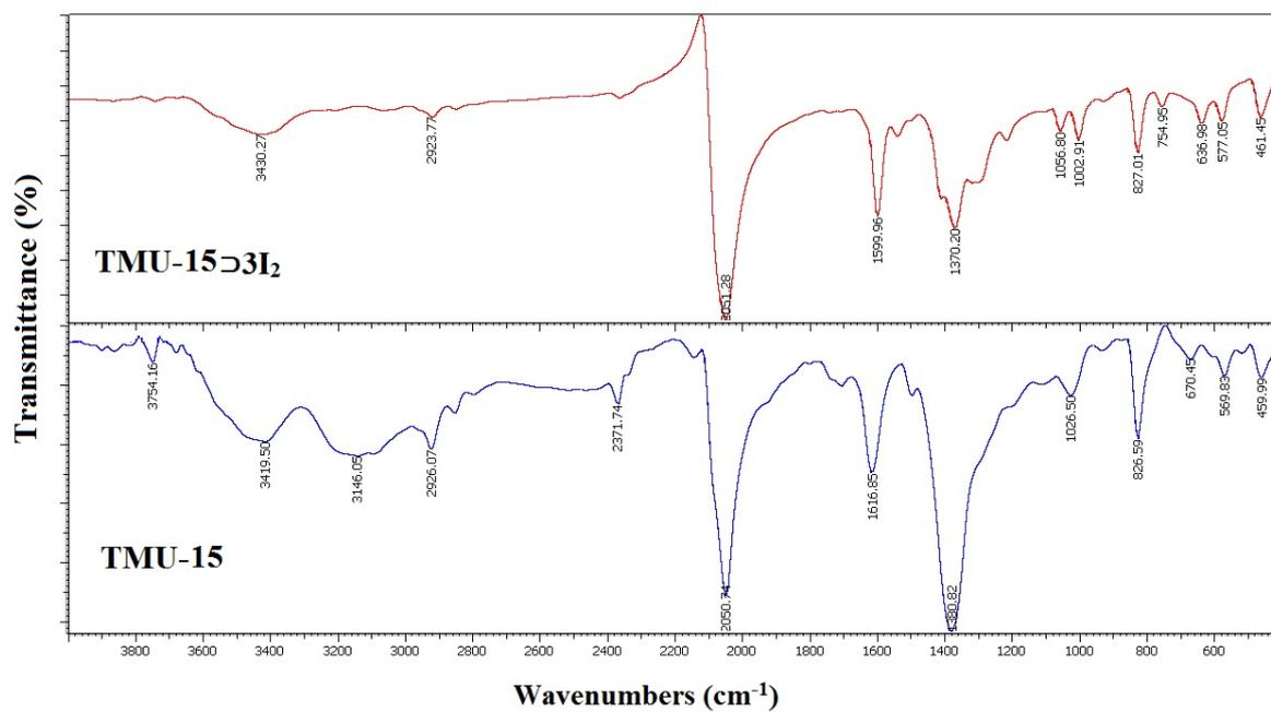
Fig. S7. The IR spectra of bulk materials as synthesized of compounds TMU-15 and TMU-15⊃3I<sub>2</sub>.
