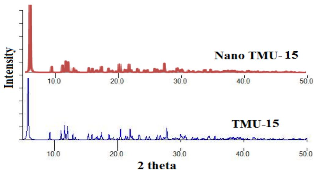
**Fig. S5.** XRD patterns of simulated based on single crystal data of compounds **TMU-15** and nano-**TMU-15** prepared by sonochemical process.
