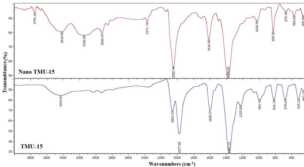
**Fig. S6.** The IR spectra of bulk materials as synthesized of compounds **TMU-15** and nano-sized compounds **TMU-15** prepared by sonochemical method.
