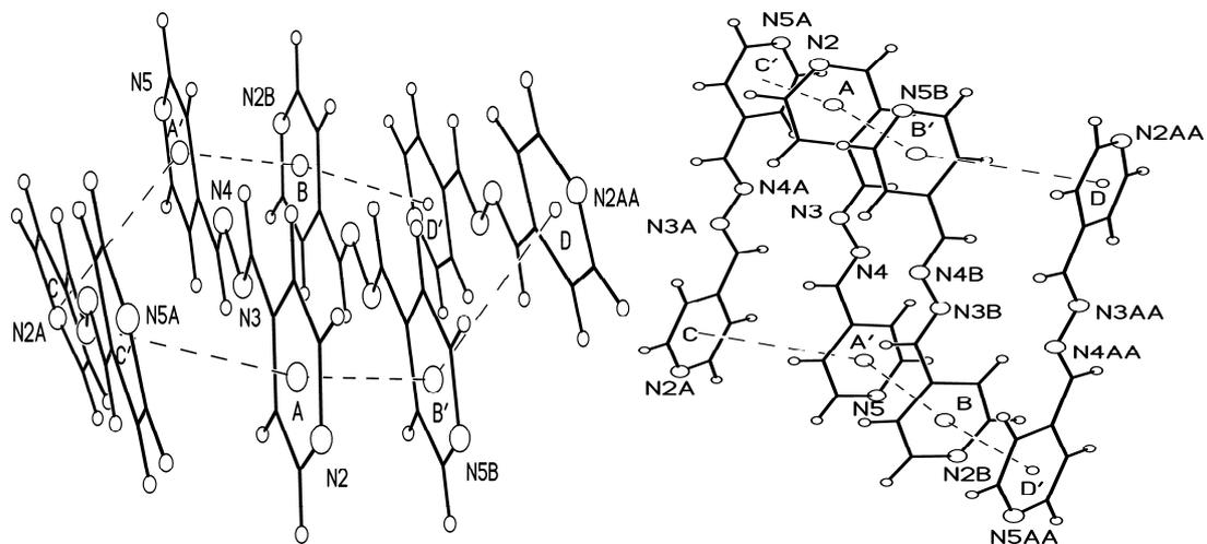
**Fig. S4.** Fragment of  $\pi$ -stacking ( $C_{10}H_{10}N_4$ ) ligands (the stacks are parallel with the crystallographic axis  $a$ ). The angle between the meanplanes of pyridine moieties and the distance between their centres for the pairs of cycles denoted A and B', B and D', A' and C are equal to, respectively,  $8.3^\circ$  and  $3.58\text{\AA}$ ; that for the A' and B, B' and D, A and C' cycles - to  $7.0^\circ$  and  $3.78\text{\AA}$ .
