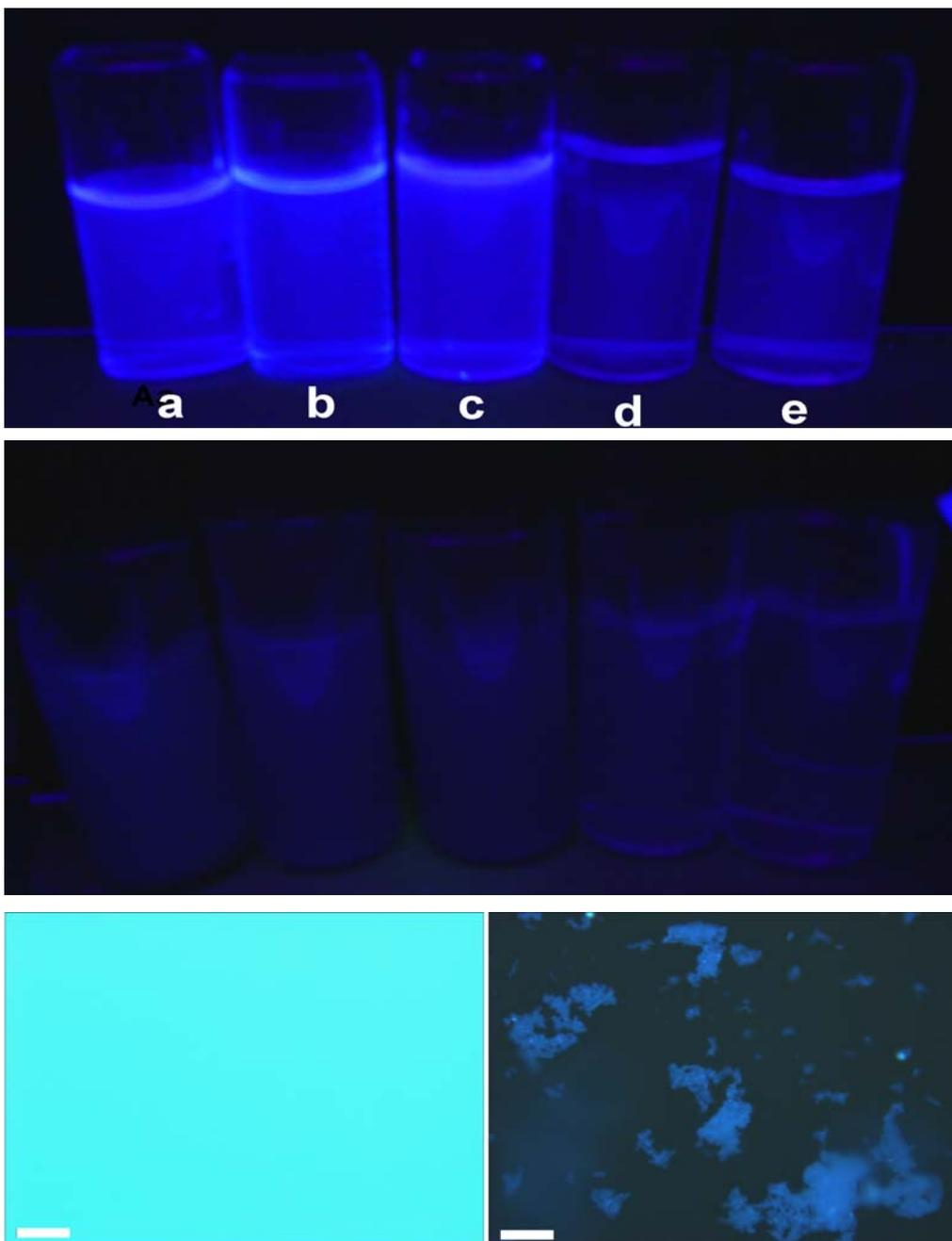
**Fig. S8.** Concentration dependent fluorescence images under a UV lamp at 365 nm. (Top) SDB solution in THF (30 mM, 10 mM, 0.5 mM, 5  $\mu$ M, 0.05  $\mu$ M), (Middle) SDB raw powder dispersed in water. (Bottom) Fluorescence images obtained by MF30 fluorescence microscope. SDB solution in THF (left), SDB raw powder dispersed in water (right), a droplet of solution or suspension was placed onto glass substrate and then subjected to observation immediately. Scale bar = 500  $\mu$ m.
