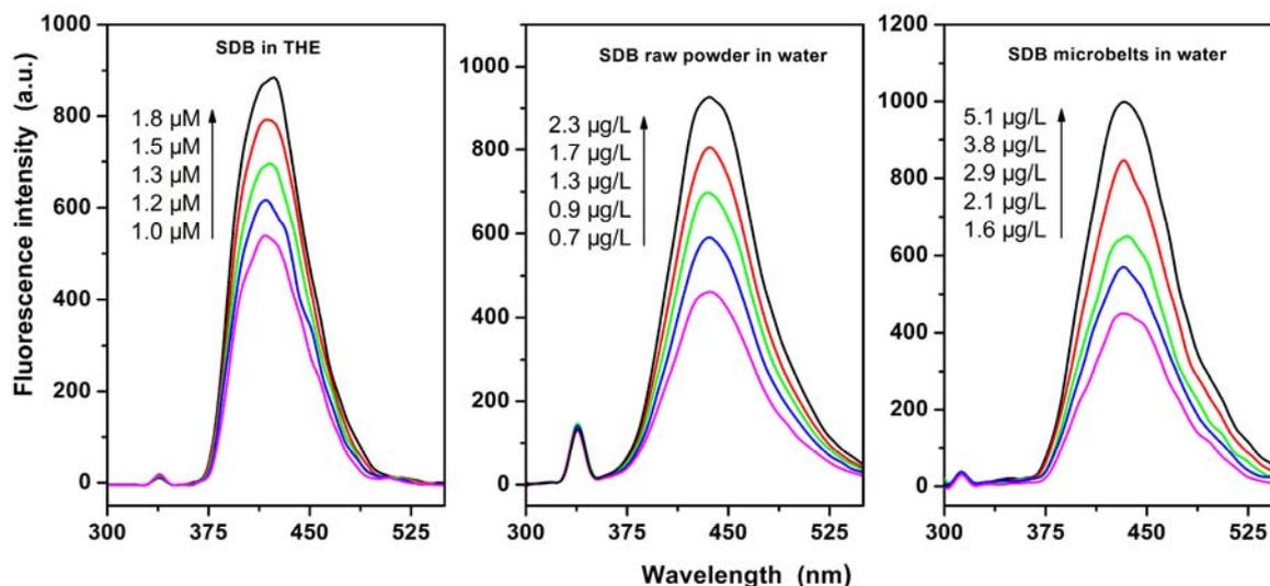
**Fig. S7.** Concentration dependent fluorescence spectra of SDB solution in THF, SDB raw powder dispersed in water, and SDB microbelts (with length of about 5 mm) dispersed in water.
