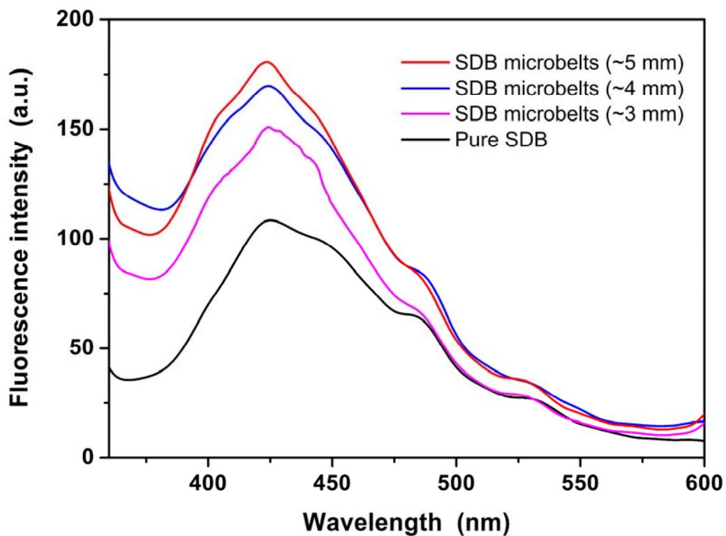
**Fig. S9.** Solid state fluorescence spectra of SDB monomer and SDB microbelts. The sample was prepared by spin coating SDB solution in THF or SDB microbelts suspension in water onto clear quartz slide.
