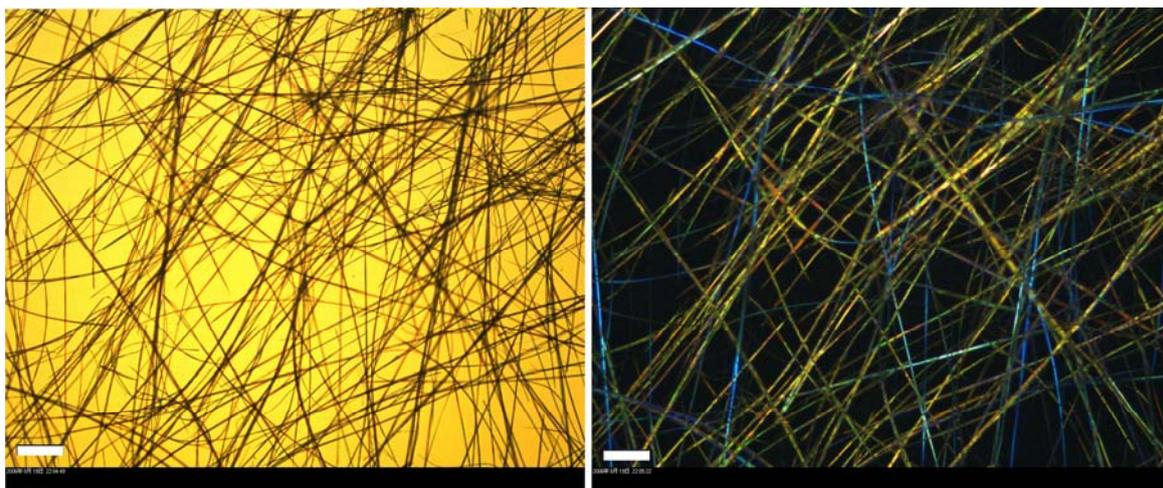
**Fig. S11.** Optical microscope (left) and polarized optical microscope (right) images of SDB microbelts prepared at SDB concentration of 3 mM. The apparent length of microbelts reaches several millimeter and endless fibers were detected under the visual field.
