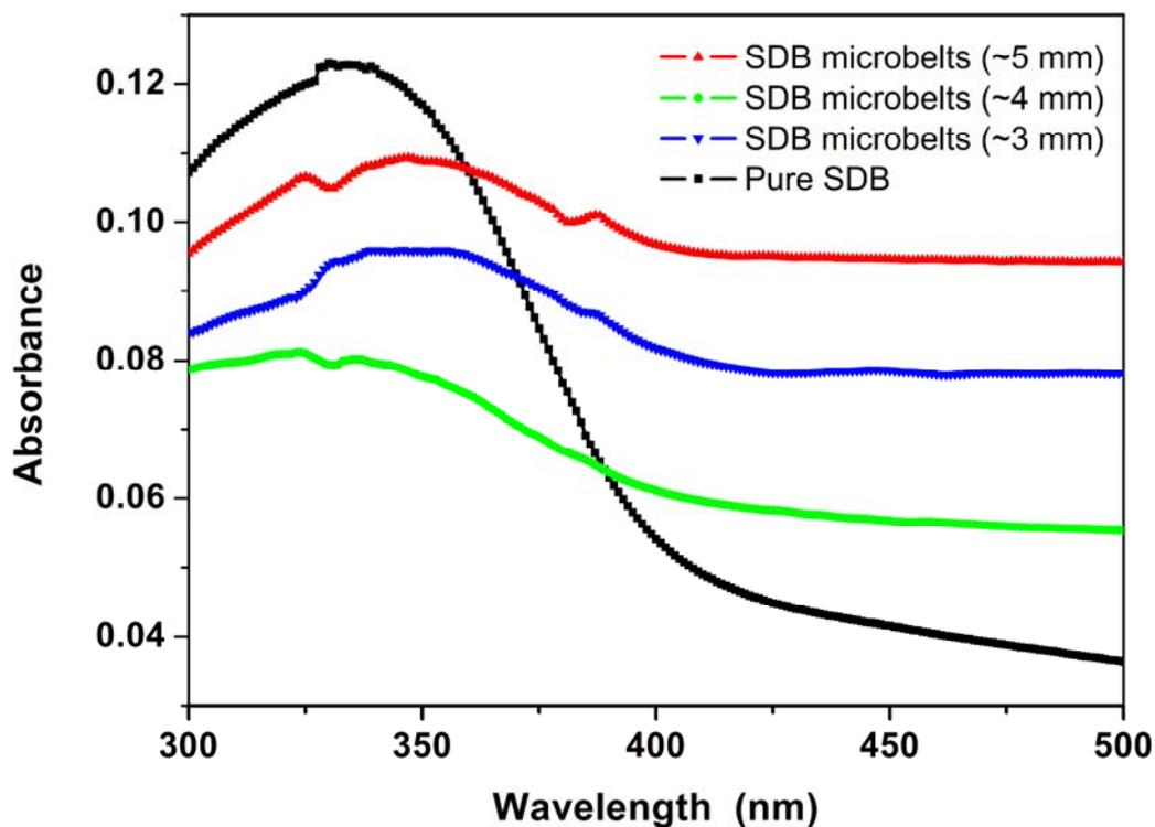
**Fig. S6.** Solid state UV-vis spectra of SDB monomer and SDB microbelts. The sample was prepared by spin coating SDB solution in THF or SDB microbelts suspension in water onto clear quartz slide.
