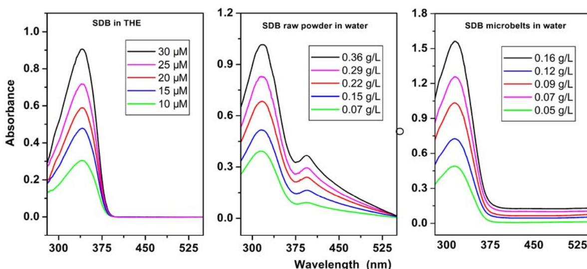
**Fig. S5.** Concentration dependent UV-vis spectra of SDB solution in THF, SDB raw powder dispersed in water, and SDB microbelts (with length of about 5 mm) dispersed in water.
