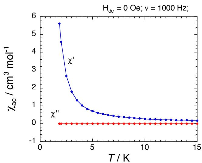
Fig. S13 Temperature dependence below 15 K of the in- and out-of-phase components of ac susceptibility for **3** at 1000 Hz with an amplitude of the ac field of 3 Oe.
