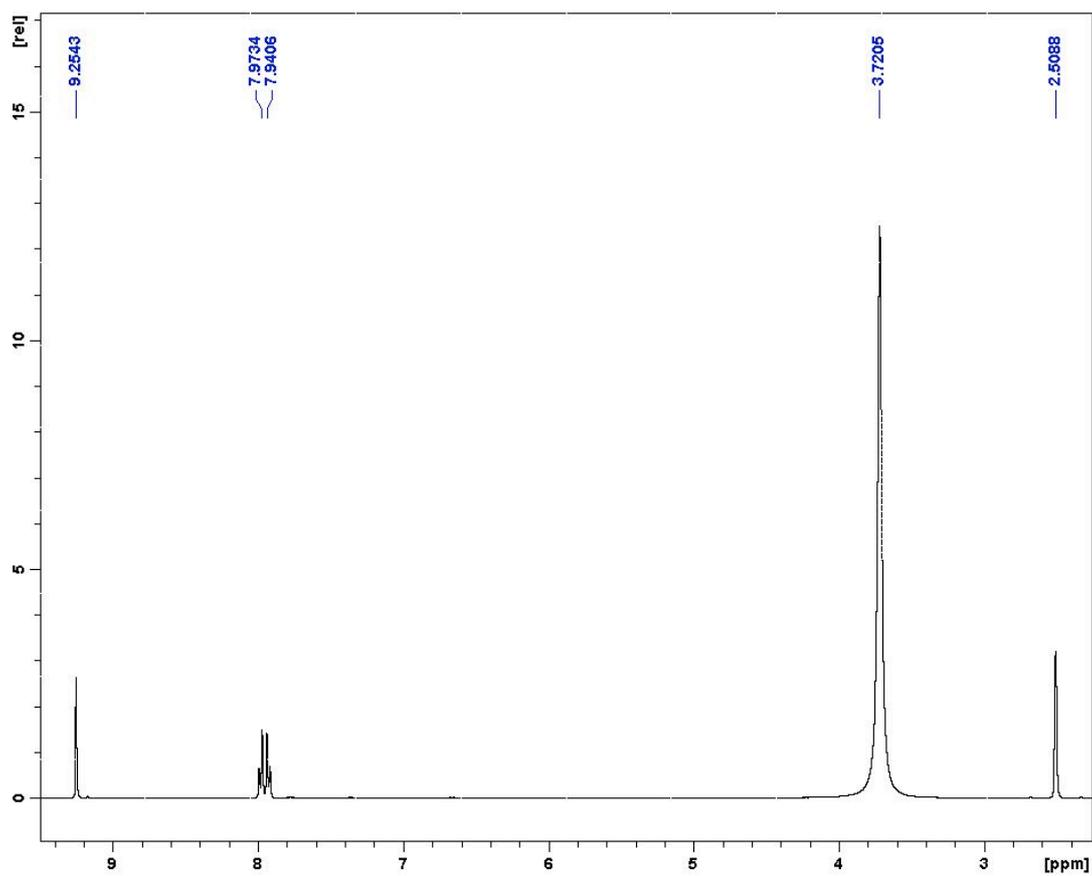
Fig. S9  $^1\text{H}$  NMR of  $\text{H}_2\text{TPAA}$  in  $\text{DMSO-d}_6$ . The strong peak at 3.7205 ppm should be  $^1\text{H}$  peak of water which could be caused by the recrystallization of  $\text{H}_2\text{TPAA}$  from water. 2.5088 ppm is the  $^1\text{H}$  peak of  $\text{DMSO-d}_6$ .
