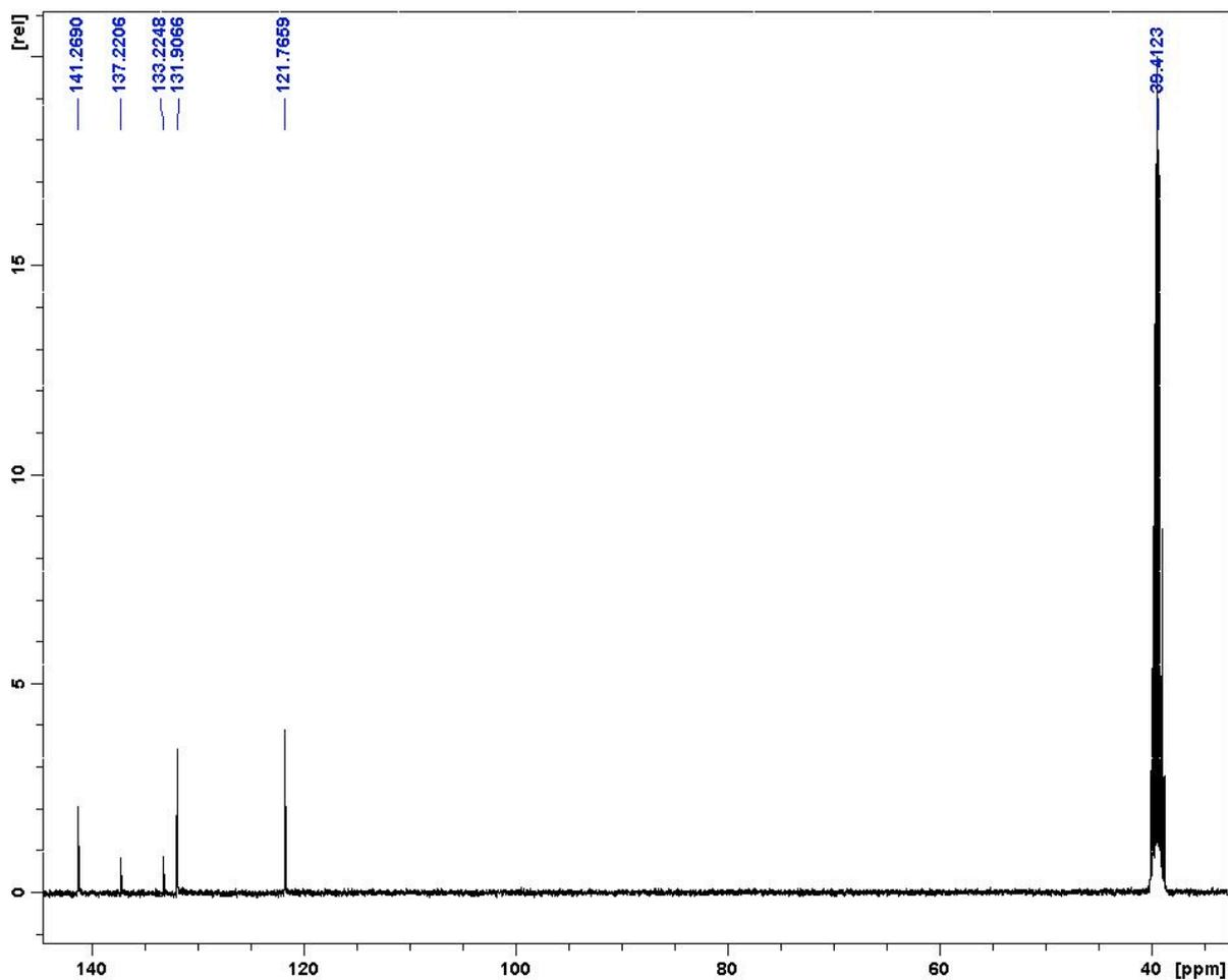
Fig. S10  $^{13}\text{C}$  NMR of  $\text{H}_2\text{TPAA}$  in  $\text{DMSO-d}_6$ . The strong peak at 39.4123 ppm is the  $^{13}\text{C}$  NMR peak of  $\text{DMSO-d}_6$ .
