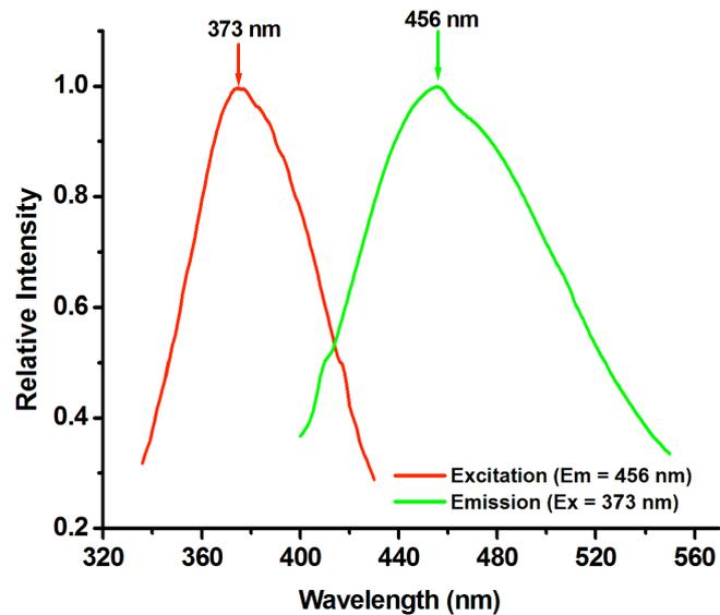
Fig. S7 Photoluminescent spectra of ligand H<sub>2</sub>TPAA in the solid state at room temperature.
