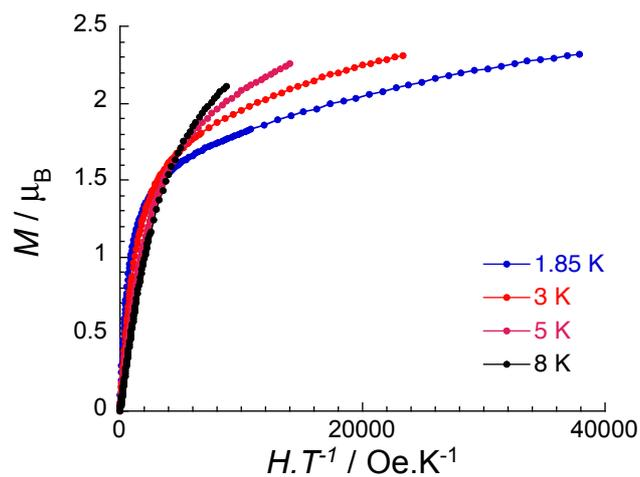
Fig. S12 Field dependence of reduced magnetization at the temperatures indicated for **3**.
