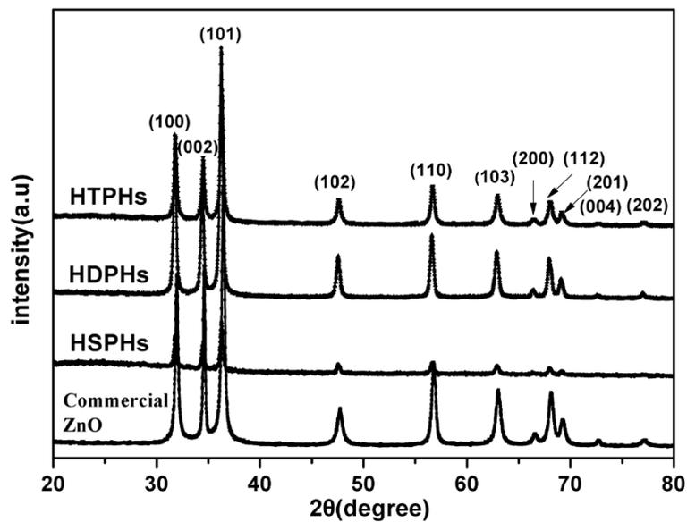
Fig.S3 XRD patterns of the as-prepared hierarchical multi-shelled ZnO porous hollow spheres and commercial ZnO.
