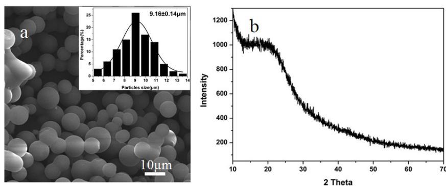
**Fig.S2 SEM (a) and XRD pattern (b) of the zinc precursor-carbon microspheres composites**
