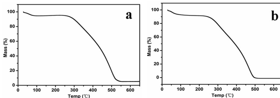
**Fig. S6** TG curves of the zinc precursor-carbon microspheres composites obtained at different heating rates: (a) heating rate of 5°C/min and (b) heating rate of 2°C/min.
