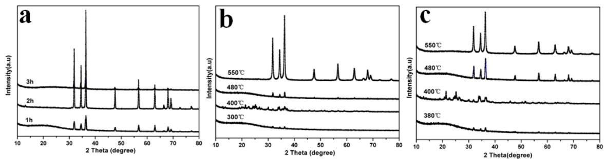
**Fig. S5** XRD patterns of the zinc precursor-carbon microspheres (a) calcined directly at 550°C for 1h, 2h and 3h, respectively, (b) calcined at a heating rate of 5°C/min to 300°C, 400°C, 480°C, and 550°C for 3 hours, respectively. (c) The zinc precursor-carbon microspheres were calcined at a heating rate of 2°C/min to 300°C, 400°C, 480°C, and 550°C for 3 hours, respectively.
