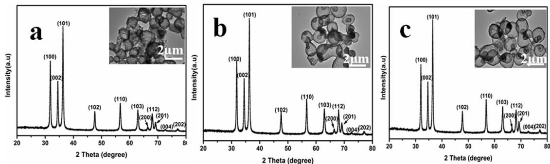
**Fig. S8** XRD results (a, b, c) and TEM images (insets in Fig. a, b and c) of hierarchical single-, double- and triple-shelled ZnO porous hollow spheres after the fifth photocatalysis experiment, respectively.
