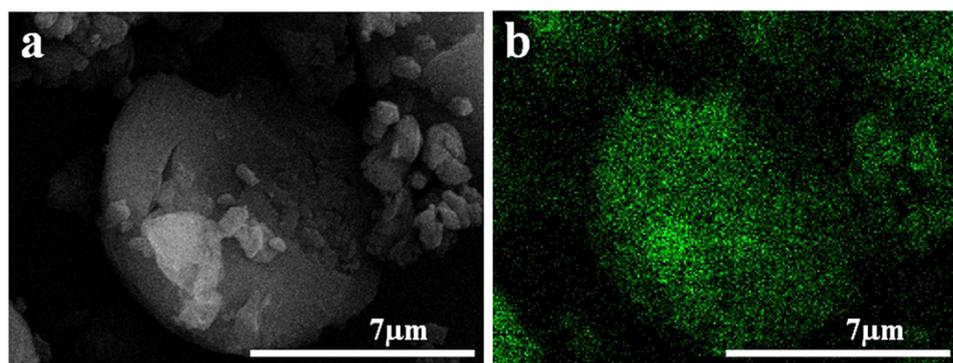
**Fig.S1 FE-SEM (a) and FE-SEM-EDX mapping (b) of the carbon microspheres after soaking in zinc sulphate solution (green indicates Zn). Note: FE-SEM and FE-SEM-EDX mapping images are at the same magnification.**
