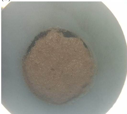
Fig. S9 The images of 1-GCE (a) and 2-GCE (b) before and after electrolysis at -1.1V vs SCE.
