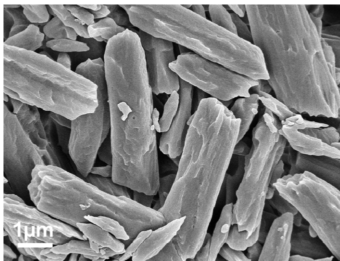
Figure S3. MOP-18 rods recrystallized in pure DMF solution and cooled in ice bath
