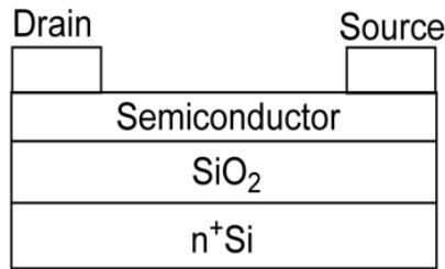
**Fig.1.** Schematic diagram of the configuration of an OTFT device.
