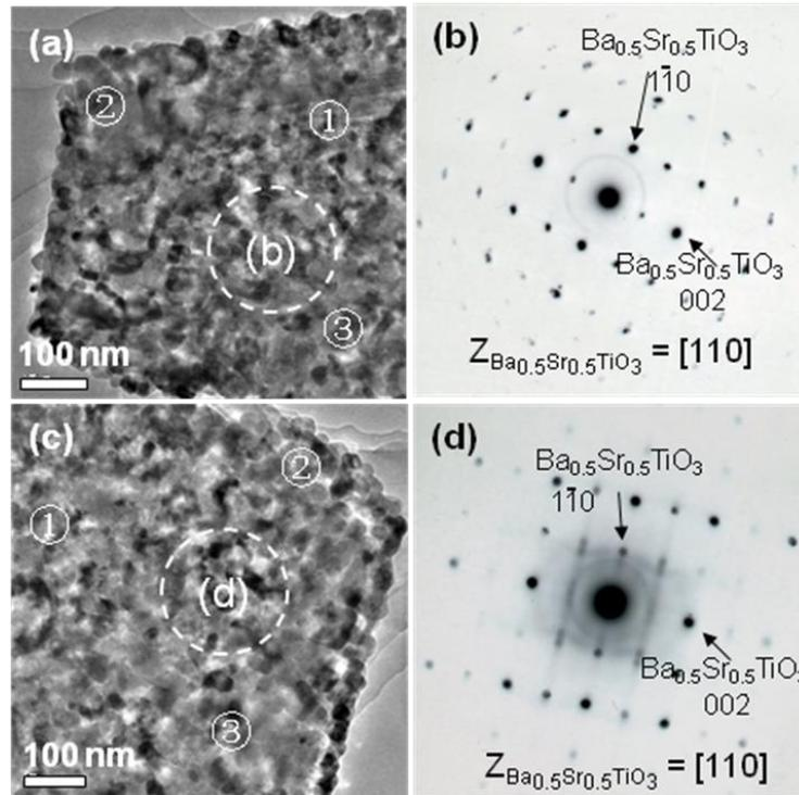
**Fig. S4†.** (a, c) TEM images and (b, d) SAED patterns of (a, b) BST-5/25-30/0 and (c, d) BST-30/0-10/20 samples obtained by solvothermal treatments of  $\text{Sr}(\text{OH})_2$  and BT/HTO nanocomposites at 200 °C for 12 h.
