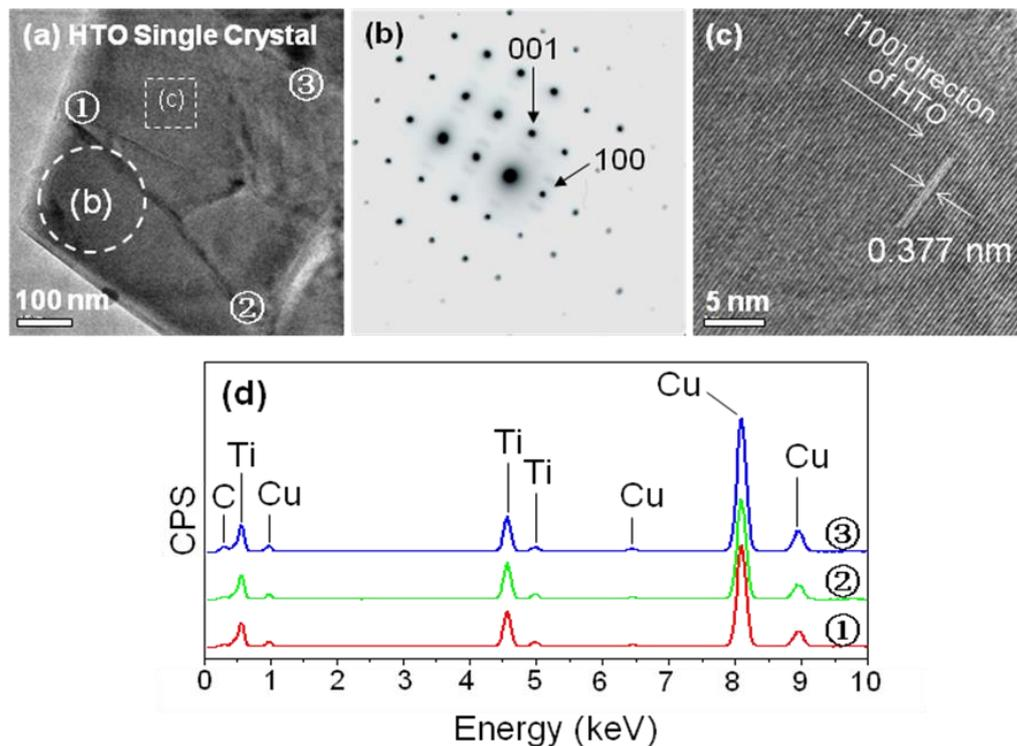
**Fig. S2†.** (a) TEM image, (b) SAED pattern, (c) HRTEM image, and (d) EDS spectra of HTO single crystal. EDS spectra ①, ② and ③ correspond to those at the positions marked ①, ②, and ③ in (a) TEM image, respectively.
