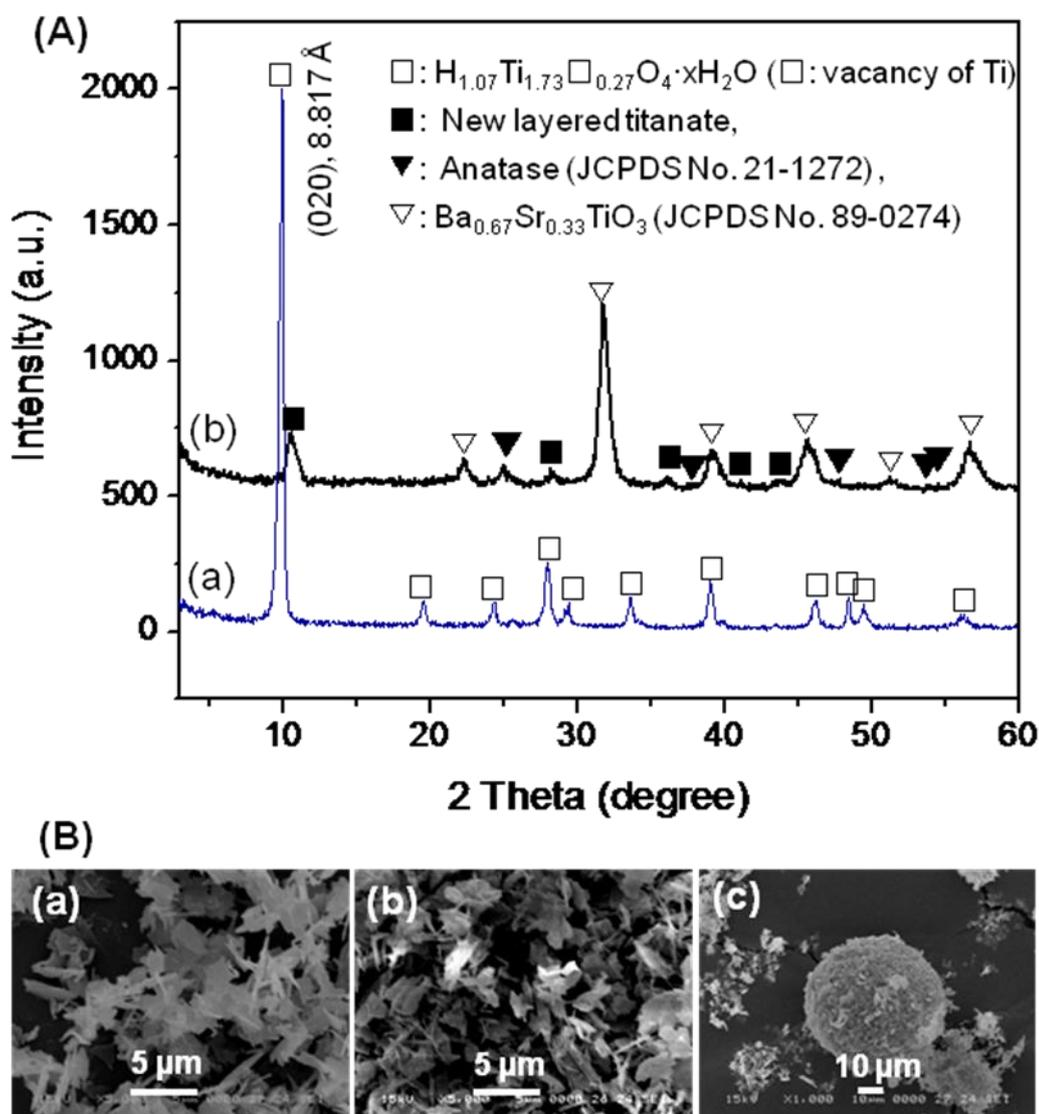
**Fig. S1†.** (A) XRD patterns and (B) SEM images of (a)  $\text{H}_{1.07}\text{Ti}_{1.73}\square_{0.27}\text{O}_4 \cdot x\text{H}_2\text{O}$  ( $\square$ : vacancy of Ti) (HTO) crystals and (b, c) samples obtained by solvothermal treatments of HTO- $\text{Ba}(\text{OH})_2$ - $\text{Sr}(\text{OH})_2$  (molar ratio of Ti/Ba/Sr = 1:0.5:0.75) mixture in water-ethanol mixed solvent (volume ratio = 5:25) at 200 °C for 12 h.
