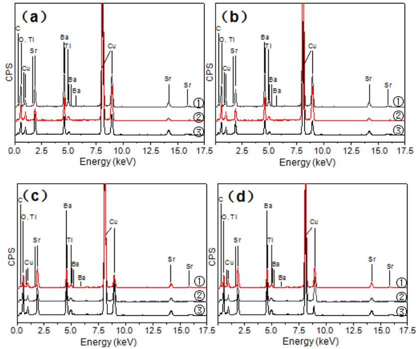
**Fig. S5†.** EDS spectra of (a) BST-30/0-30/0, (b) BST-5/25-30/0, (c) BST-30/0-10/20, and (d) BST-5/25-30/0 samples corresponding to the TEM images of Fig. 4a, S4a, S4c, 4c, respectively. EDS spectra of labeled “①”, “②”, and “③” symbol correspond to optionally selected positions in platelike particles shown in TEM images of Fig. 4a, S4a, S4c, 4c, respectively.
