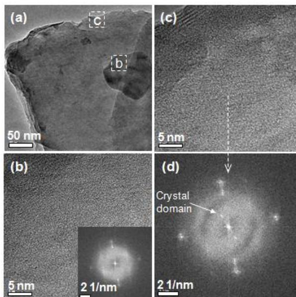
**Fig. S3†** (a) TEM image and (b, c) HRTEM images of BHA-30/0 sample obtained by solvothermal treatment of HTO single crystals and  $\text{Ba}(\text{OH})_2$  (molar ratio of Ti/Ba = 2) in water solvent at 150 °C for 12 h. (b, c) HRTEM images are derived from the (b, c) white panes in (a) TEM image, respectively. The inserted FFT pattern in (b) TEM image and (d) FFT pattern are derived from whole region of (b, c) HRTEM images by Fast Fourier Transformation, respectively.
