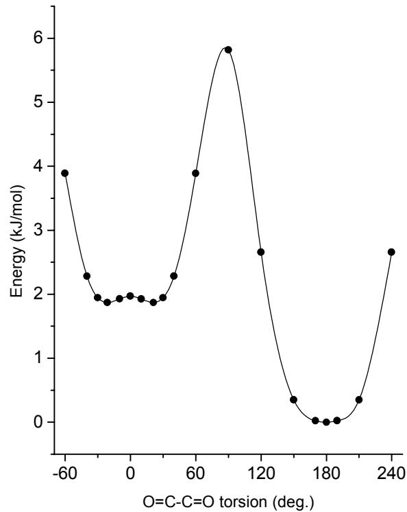
Fig. S1. Electronic energy of DMO calculated at MP2/6-31G\*\* level as a function of O=C-C=O torsion.
