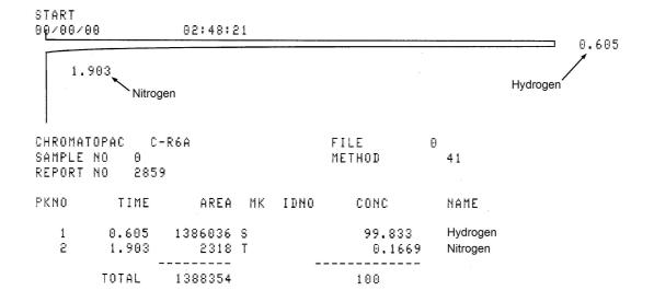
Data of the gas chromatography obtained from the bubbles on the negative AFM tip during 1-butanol polymerization. Only the ratio of the concentration of hydrogen and nitrogen is addressed in this data, since the machine was not suitable for detecting all the gasses produced during the 1-butanol polymerization. Gas chromatography detected the hydrogen concentration to be 99 times more dense than nitrogen. Gas chromatograph, GC-14BPTF, Shimadzu.
