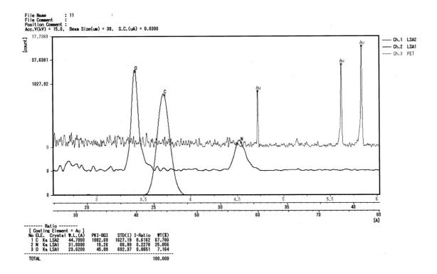
Electron Probe Microanalysis (EPMA) revealed that 1-butanol polymer on an AFM tip contained 25 weight percent of nitrogen, 67.8 weight percent of carbon, and 7.2 weight percent of oxygen. The ratio of the number of atoms per unit mass is 12 : 4 : 1 for carbon : nitrogen : oxygen. The data demonstrated that nitrogen molecules in air were fixed to 1-butanol polymer. AFM tip, DF-20 (Au-coated silicon tip) SII.
