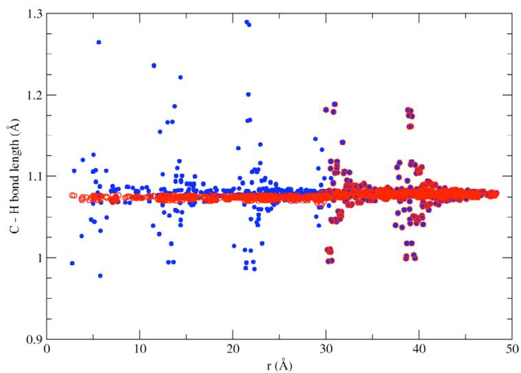
**Figure S5:** C-H bond lengths around dislocated paracetamol before and after atomic relaxation of the core. Blue circles show the bond lengths after introduction of the dislocation assuming the crystal is a homogeneous linear elastic solid, red open circles show the bond lengths after atomistic relaxation of all atoms within 30 Å of the core to an energy minimum.
