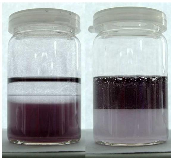
FIGURE S4. Photographs of glass vials containing aqueous solutions (bottom) of 4-MBA-capped Au nanocrystals with a mean size of 6 nm in contact with heptane (top), after implementation of pH-switched self-assembly of the nanocrystals at the water/heptane interface 4 times. In the left glass vial, the pH of the aqueous solution of the nanocrystals was 9, while in the right vial, the pH was 2.
