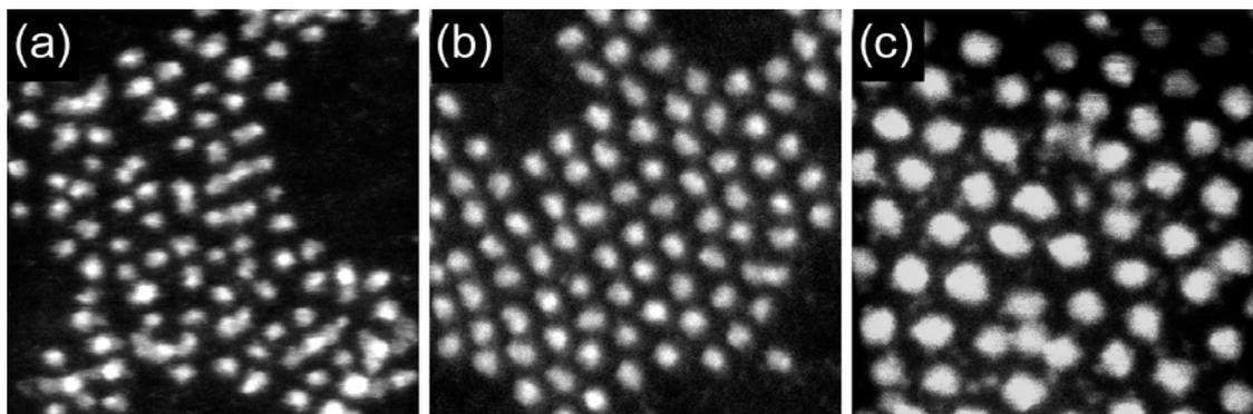
**Figure S1.** Scanning transmission electron micrographs of PbS QDs with average diameters  $3.2 \pm 0.5$  (a),  $3.8 \pm 0.4$  (b), and  $5.4 \pm 0.7$  nm (c).
