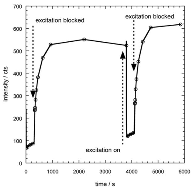
**Figure S2.** Fluorescence intensity time trace of 5.4-nm PbS QDs exhibiting a complete recovery of initial intensity levels after sitting in darkness for ~10 min. The beginning of excitation and recovery are marked on the plot and are cycled a total of two times.
