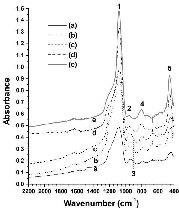
**Figure S2.** FTIR spectral evolution after deposition of (a) Au-doped film (first layer) dried at 60 °C, (b) Pt-doped film onto the first layer and dried at 60 °C, (c) after UV-treatment of 2L film, and subsequent heat-treated TL film in air: (d) 450 °C and (e) 550 °C for 1 h. Films were deposited on double side polished (intrinsic, IR transparent) Si wafers.
