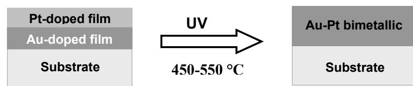
**Figure S1** Schematic representation of the two-layer (2L) film assembly before and after UV/thermal treatments
