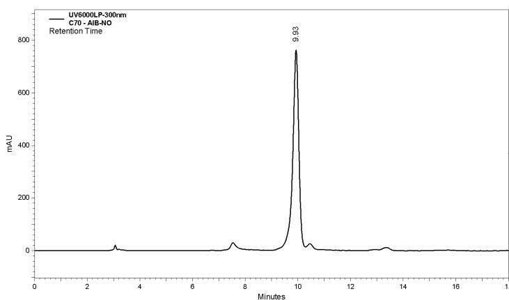
**Figure S5.** HPLC trace of **1a-c** (Phenomenex Luna SiO<sub>2</sub>, 5μ, 250 × 4.6 mm; toluene/ethyl acetate 9:1, 1ml/min; λ = 300 nm).
