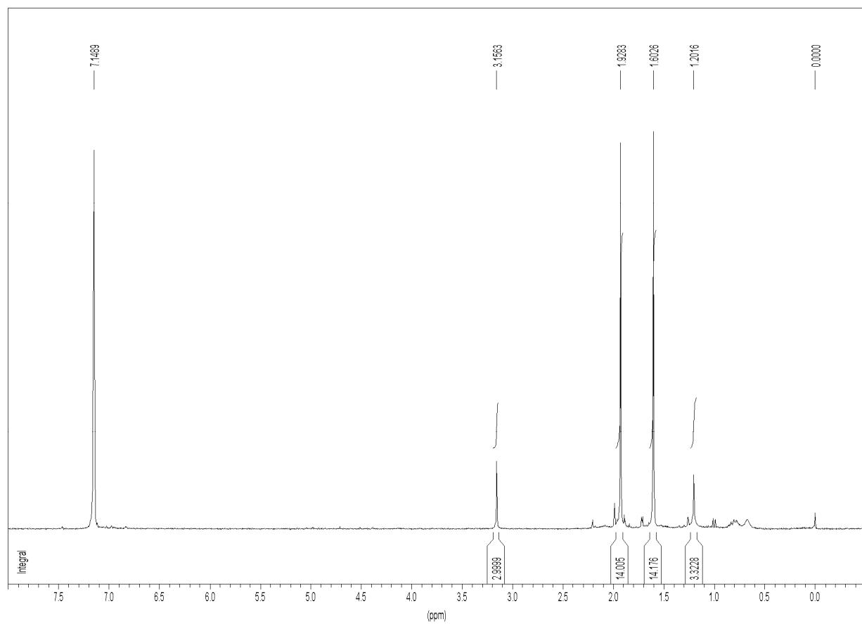
**Figure S2.** <sup>1</sup>H NMR spectrum of **2a-c** (250MHz, CS<sub>2</sub>/benzene-C<sub>6</sub>D<sub>6</sub> 5:1)
