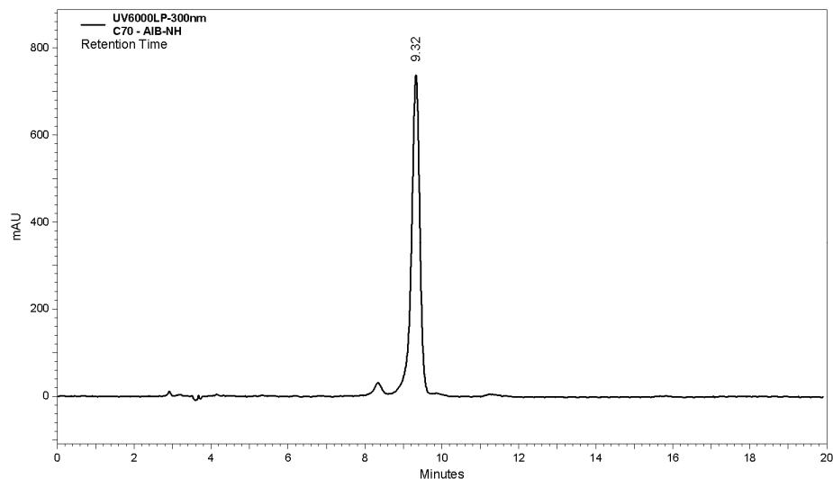
**Figure S1.** HPLC trace of **2a-c** (Phenomenex Luna SiO<sub>2</sub>, 5μ, 250 × 4.6 mm; toluene/ethyl acetate 9:1, 1ml/min; λ = 300 nm).
