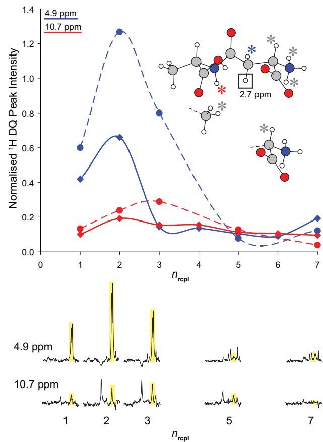
**Fig. S8** A comparison of simulated (solid lines, diamonds, SPINEVOLUTION) and experimental (dashed lines, circles, 500 MHz, 12.5 kHz)  $^1\text{H}$  DQ build-up curves for DQCJs at the  $\text{CH}_2(\text{b})$  SQ frequency.
