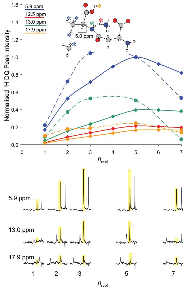
**Fig. S10** A comparison of simulated (solid lines, diamonds, SPINEVOLUTION) and experimental (dashed lines, circles, 500 MHz, 12.5 kHz)  ${}^1\text{H}$  DQ build-up curves for DQCs at the  $\text{CH}(\text{Ala})$  SQ frequency.
