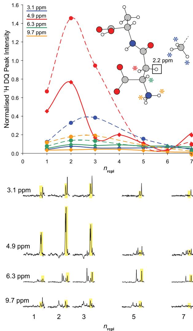
**Fig. S7** A comparison of simulated (solid lines, diamonds, SPINEVOLUTION) and experimental (dashed lines, circles, 500 MHz, 12.5 kHz)  $^1\text{H}$  DQ build-up curves for DQCs at the  $\text{CH}_2(\text{a})$  SQ frequency.
