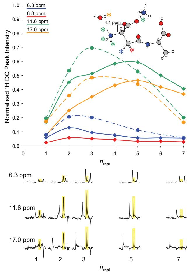
**Fig. S9** A comparison of simulated (solid lines, diamonds, SPINEVOLUTION) and experimental (dashed lines, circles, 500 MHz, 12.5 kHz)  $^1\text{H}$  DQ build-up curves for DQCs at the CH(Asp) SQ frequency.
