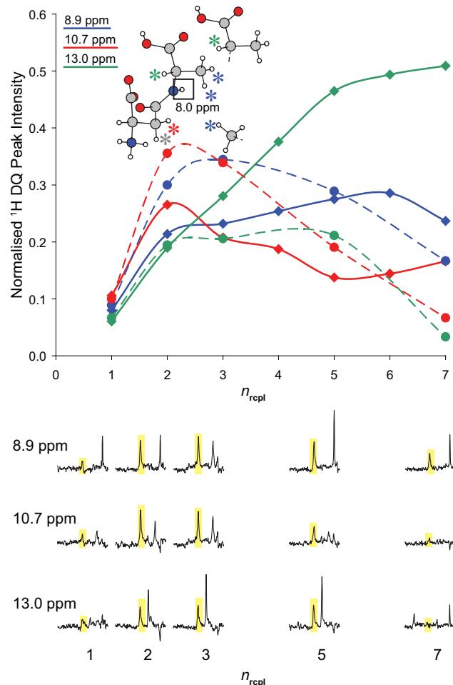
**Fig. S11** A comparison of simulated (solid lines, diamonds, SPINEVOLUTION) and experimental (dashed lines, circles, 500 MHz, 12.5 kHz)  $^1\text{H}$  DQ build-up curves for DQCs at the NH SQ frequency.
