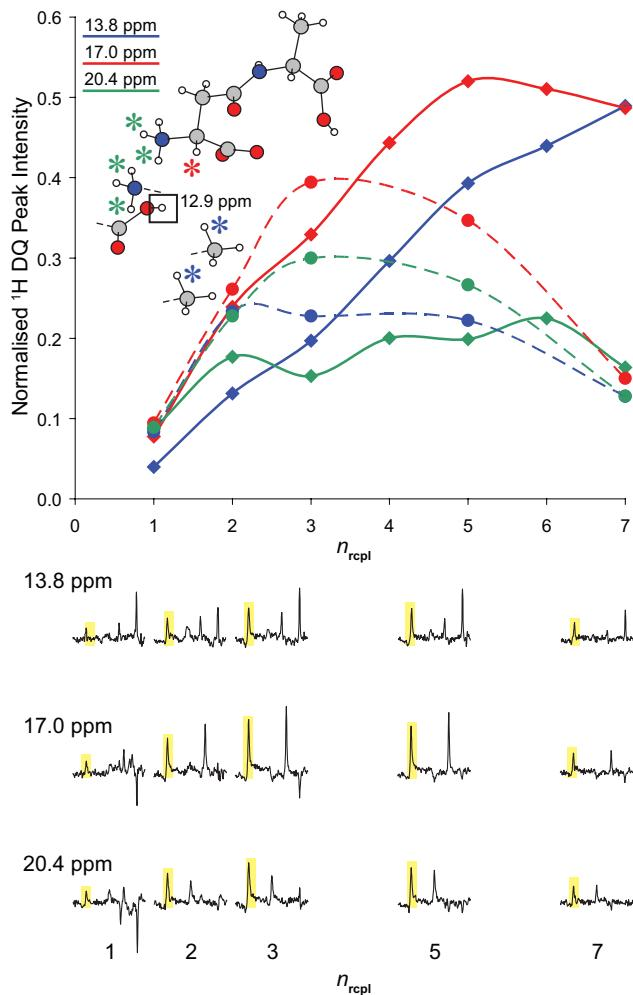
**Fig. S12** A comparison of simulated (solid lines, diamonds, SPINEVOLUTION) and experimental (dashed lines, circles, 500 MHz, 12.5 kHz)  $^1\text{H}$  DQ build-up curves for DQCs at the OH SQ frequency.
