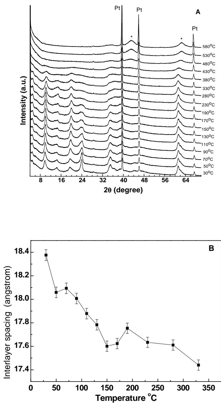
**Figure S2** *In situ* XRD patterns of PTCB intercalated Mg-Al-LDH in the temperature range 30-580 °C: (A)  $2\theta$  angular domain from 4 to 70° (\*: MgO); (B) Variation of the interlayer spacing with temperature.
