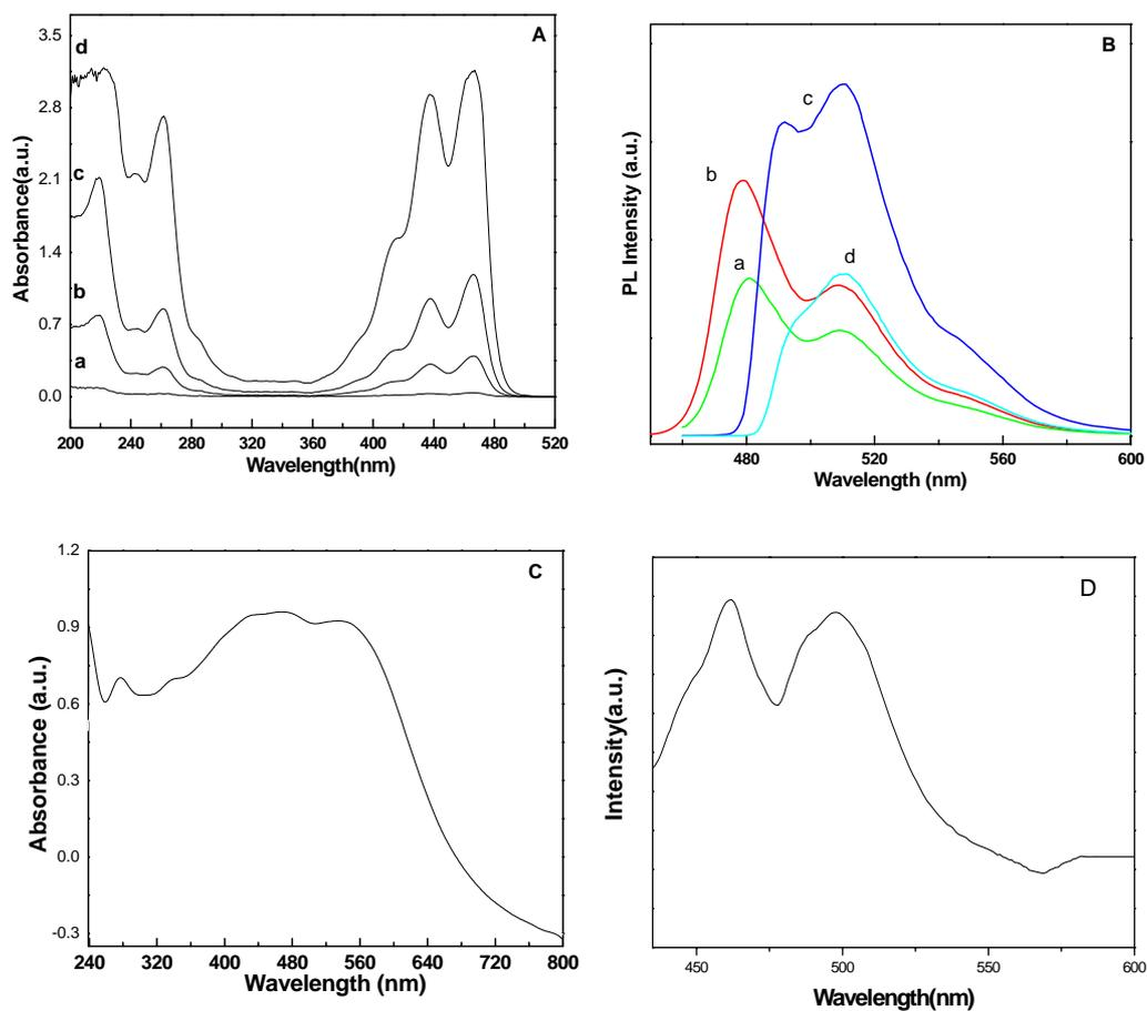
**Figure S1.** (A) UV-vis absorption spectra and (B) photoluminescence spectra of PTCB aqueous solution with various concentrations: (a) 1 μM, (b) 3 μM, (c) 10 μM and (d) 30 μM. (C) UV-Vis absorption spectra and (D) photoemission spectra of PTCB/LDH powder.
