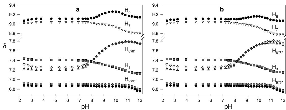
**Figure S1 :** Chemical shifts  $\delta$  from  $^1H$ -NMR titrations for NBA ( $2.0 \times 10^{-3}$  mole.L $^{-1}$ ) in the presence of 2 equivalents of  $K^+$  (a) and 2 equivalents of  $Na^+$  (b) as a function of pH at 25.0 °C (CD<sub>3</sub>OD:D<sub>2</sub>O-80:20).
