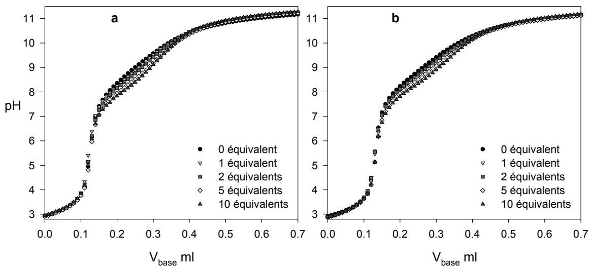
**Figure S2 :** Potentiometric titration curves of NBA ( $1.5 \times 10^{-3}$  mole.L $^{-1}$ ), without and with various concentrations of  $K^+$  (a) and  $Na^+$  (b) cations at 25.0 °C
