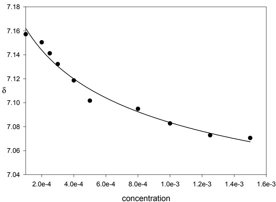
**Figure S12 :** Chemical shifts of the H<sub>3</sub> proton *vs* the NBA concentration in aqueous medium (pH = 8.3) at 25.0°C.
