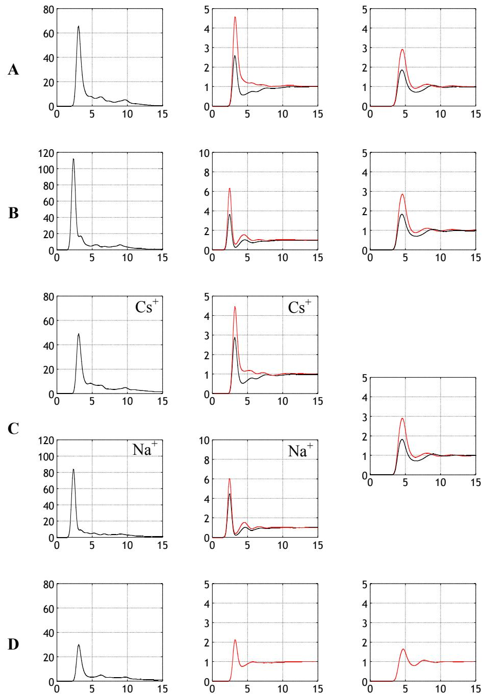
**Figure S9 : A – D** solutions: RDFs  $X^+ \cdots O_{\text{NBA}}$  (first column),  $X^+ \cdots O_{\text{wat}}$  (red, second column),  $X^+ \cdots O_{\text{MeOH}}$  (black, second column),  $N_{\text{Me4N}^+} \cdots O_{\text{wat}}$  (red, third column),  $N_{\text{Me4N}^+} \cdots O_{\text{MeOH}}$  (black, third column).
