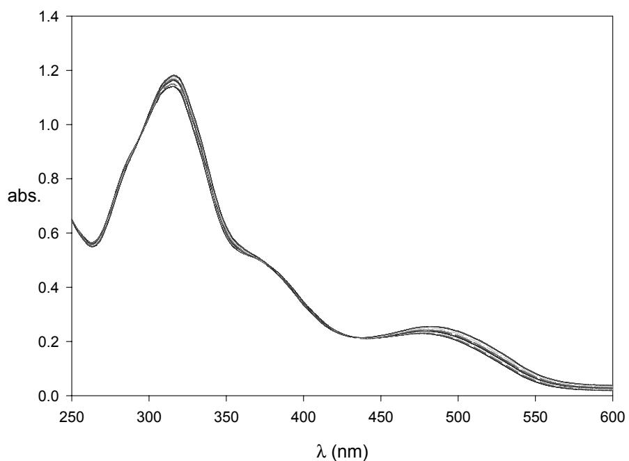
Figure S3 : UV-Visible spectra variations at pH 9.9 for various  $\text{Cs}^+$  to NBA (0 to 8) ratios.
