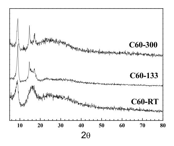
XRD diagrams of fluorinated C60 according to the fluorination temperature.
