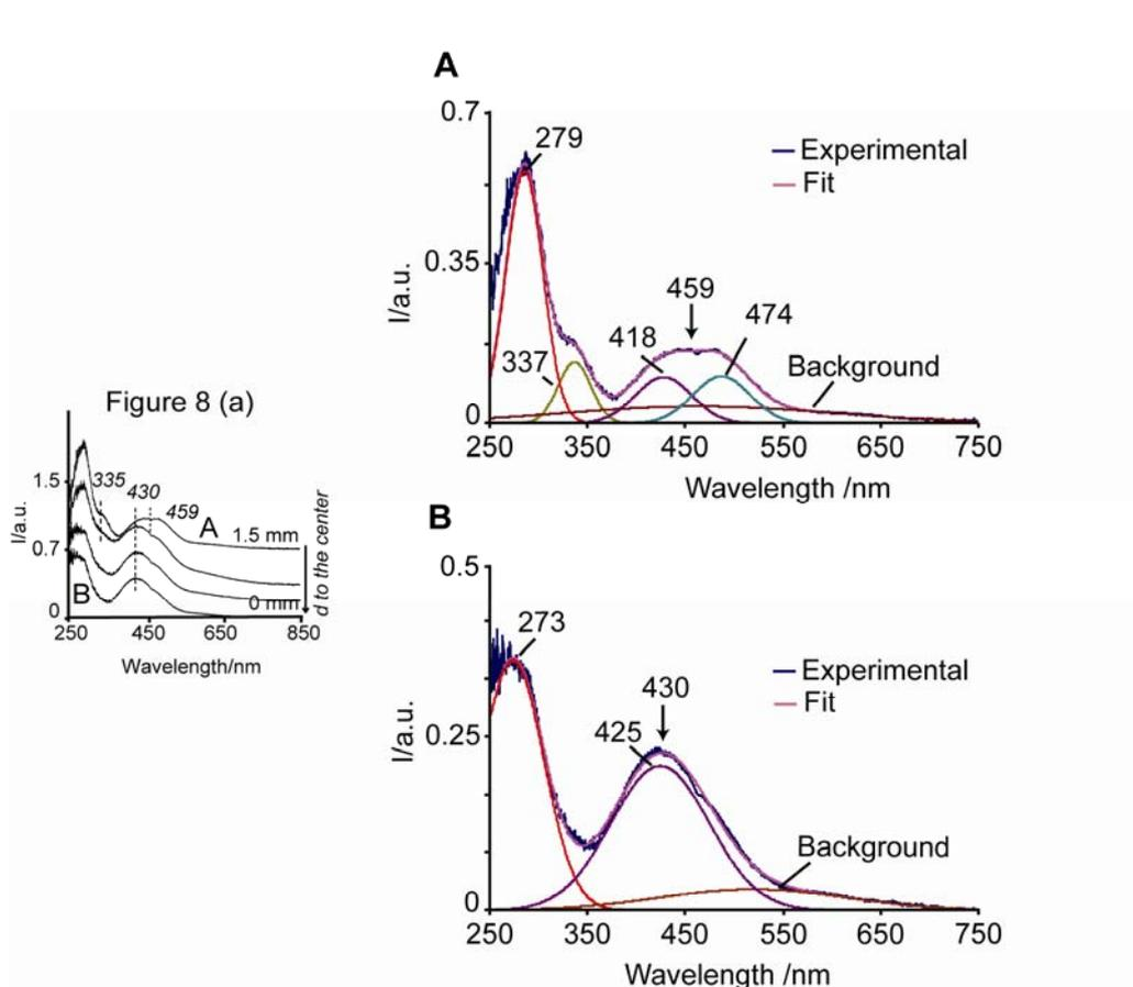
**Figure H.** Curve analysis of the UV-Vis spectra from Figure 8 (a): Space resolved UV-Vis spectra from the edge to the center of a pellet after impregnation and drying with solution 1wt%Pd-A1.
