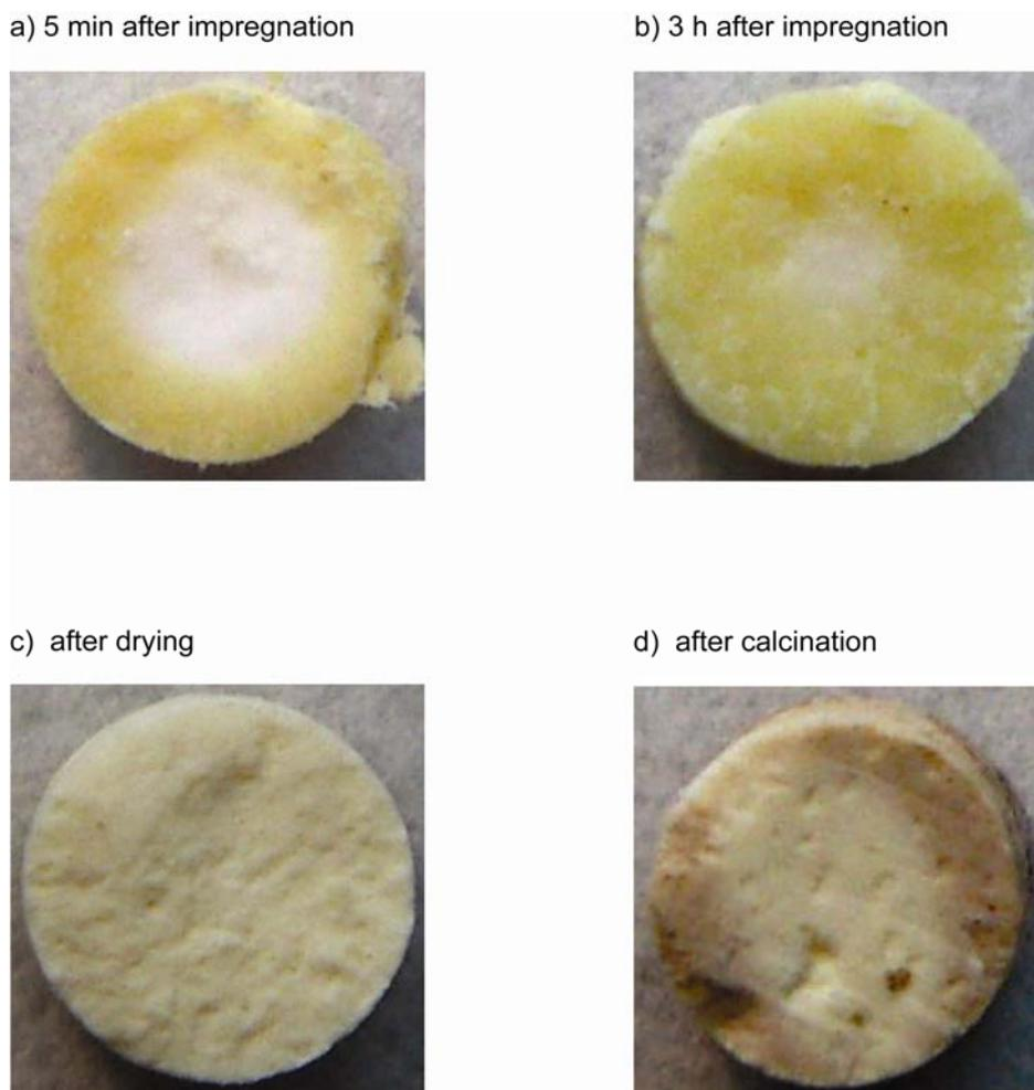
**Figure C.** Digital photographs of pellets prepared from solution 1wt%Pd-B4: (a) 5 min after impregnation; (b) 3 h after impregnation; (c) after drying; and (d) after calcination.
