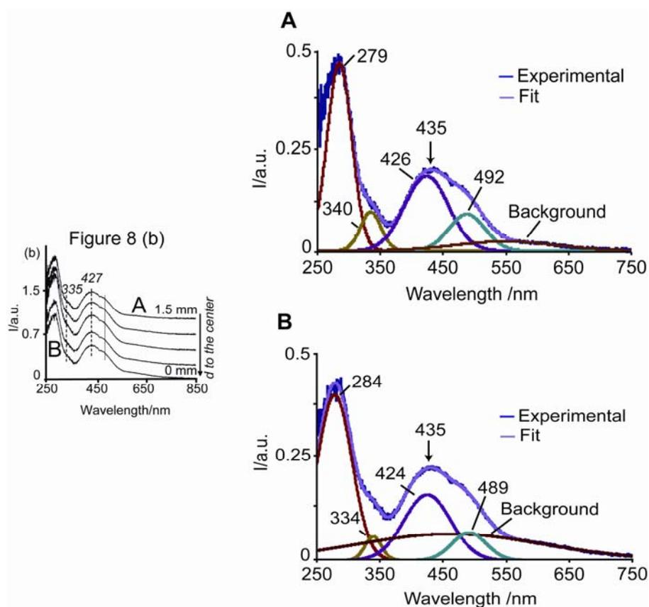
**Figure I.** Curve analysis of the UV-Vis spectra from Figure 8 (b): Space resolved UV-Vis spectra from the edge to the center of a pellet after impregnation and drying with solution 1wt%Pd-B4.
