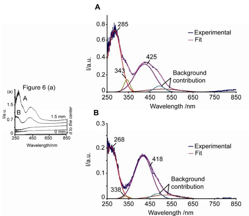
**Figure D.** Curve analysis of the UV-Vis spectra from Figure 6 (a): Space resolved UV-Vis spectra from the edge to the center of pellets 5 min after impregnation with solution 1wt%Pd-A1.
