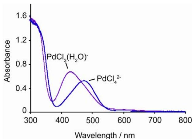
**Figure A.** UV-Vis spectra of the pure components  $\text{PdCl}_4^{2-}$  (Solution A6) and  $\text{PdCl}_3(\text{H}_2\text{O})^-$  (solution B0).
