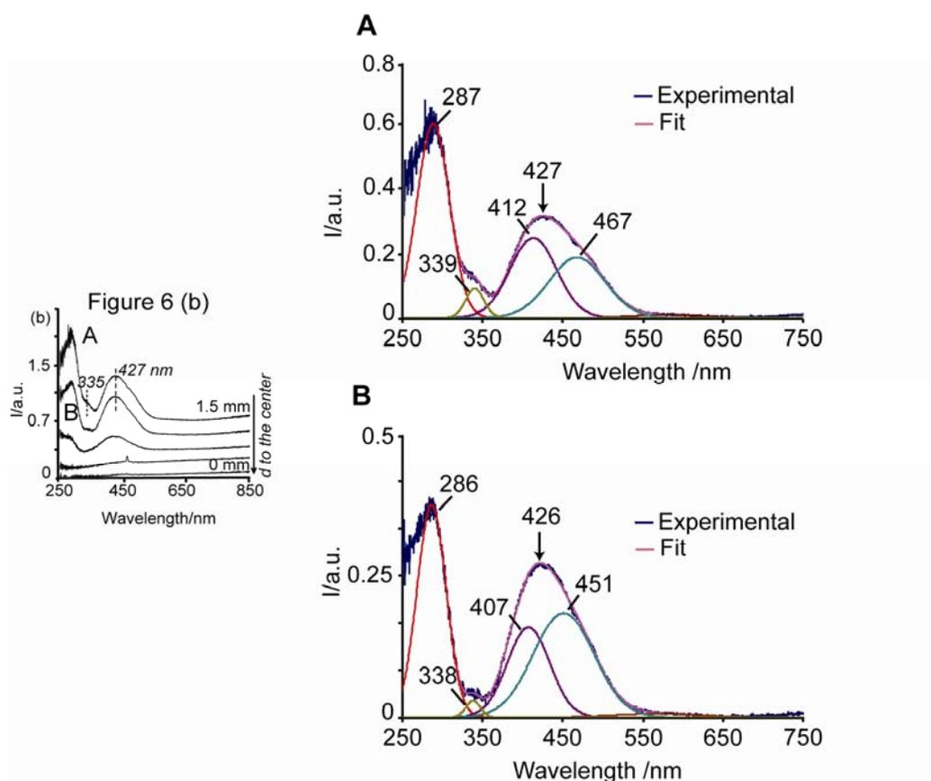
**Figure E.** Curve analysis of the UV-Vis spectra from Figure 6 (a): Space resolved UV-Vis spectra from the edge to the center of pellets 5 min after impregnation with solution 1wt%Pd-B4.
