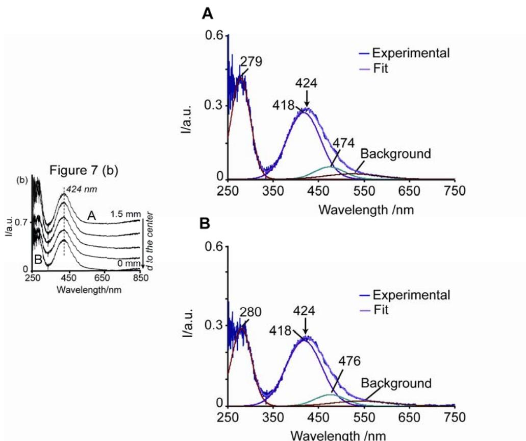
**Figure G.** Curve analysis of the UV-Vis spectra from Figure 7 (b): Space resolved UV-Vis spectra from the edge to the center of pellets 3 h after impregnation with solution 1wt%Pd-B4.
