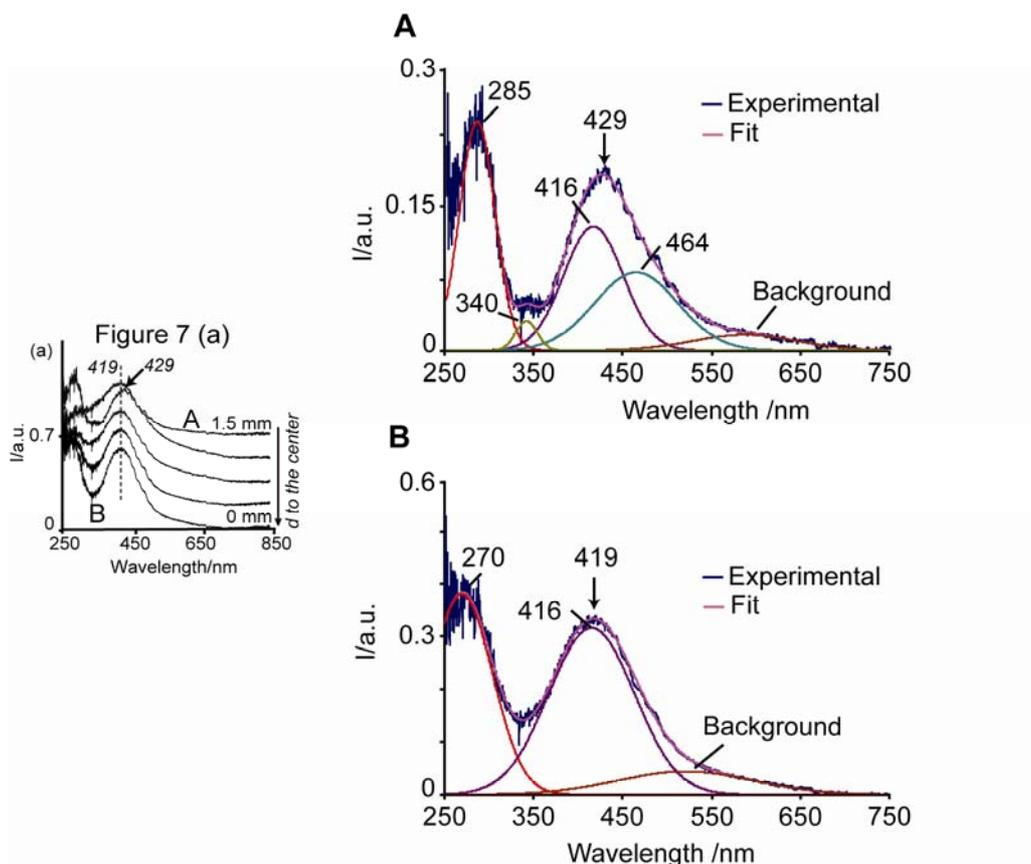
**Figure F.** Curve analysis of the UV-Vis spectra from Figure 7 (a): Space resolved UV-Vis spectra from the edge to the center of pellets 3 h after impregnation with solution 1wt%Pd-A1.
