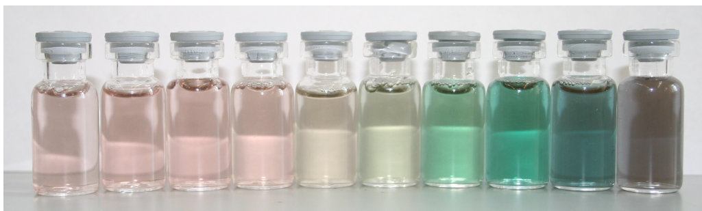
Fig. 2S. Changes in colloid colors with an increase in the mass ratio m_{\text{Ag}} / m_{\text{Au}} from 0 (left) to 1.14 (right). The initial sample is NR-800.
