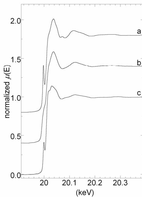
**Fig. S3.** Raw X-ray absorption spectra, collected in transmission mode at SSRL, for (a) MgMoO<sub>4</sub> (BL 4-1), (b) MgMo<sub>2</sub>O<sub>7</sub> (BL 2-3), and (c) Mo/HZSM-5 (BL 4-1).
