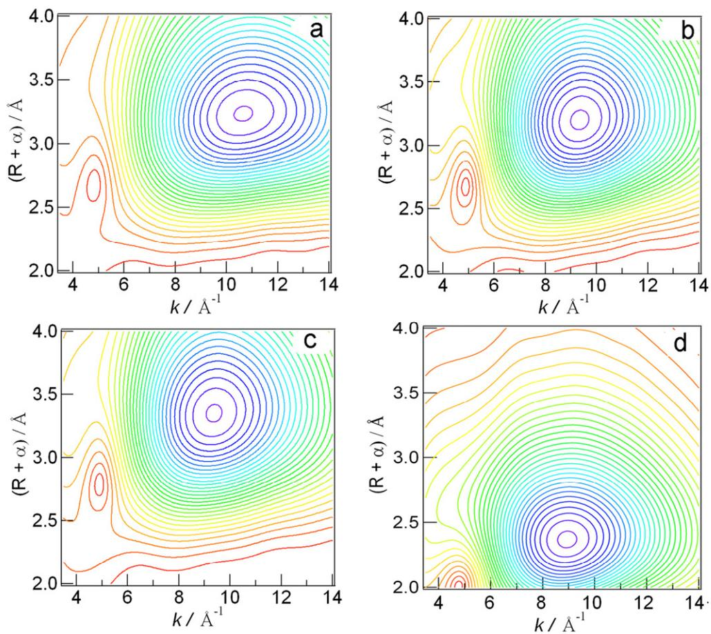
**Fig. S10.** Calculated WT plots for Mo-Mo-O paths. See Table S2 for structural parameters.
