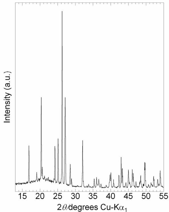
**Fig. S2.** Powder XRD pattern of MgMo<sub>2</sub>O<sub>7</sub>.
