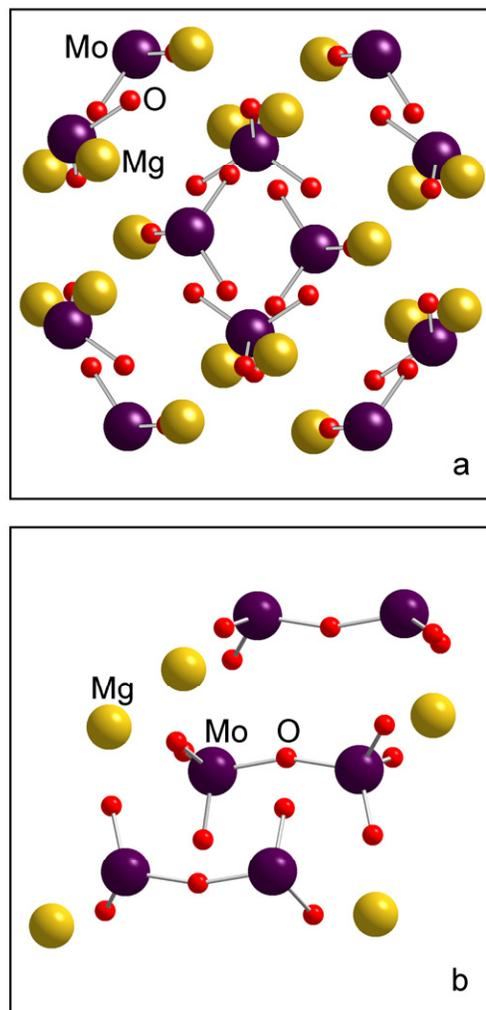
**Fig. S1.** Crystal structures of (a) MgMoO<sub>4</sub>, showing isolated MoO<sub>4</sub><sup>2-</sup> tetrahedra;<sup>1</sup> and (b) MgMo<sub>2</sub>O<sub>7</sub>, showing oxygen-bridged MoO<sub>3</sub> groups.<sup>2</sup>
