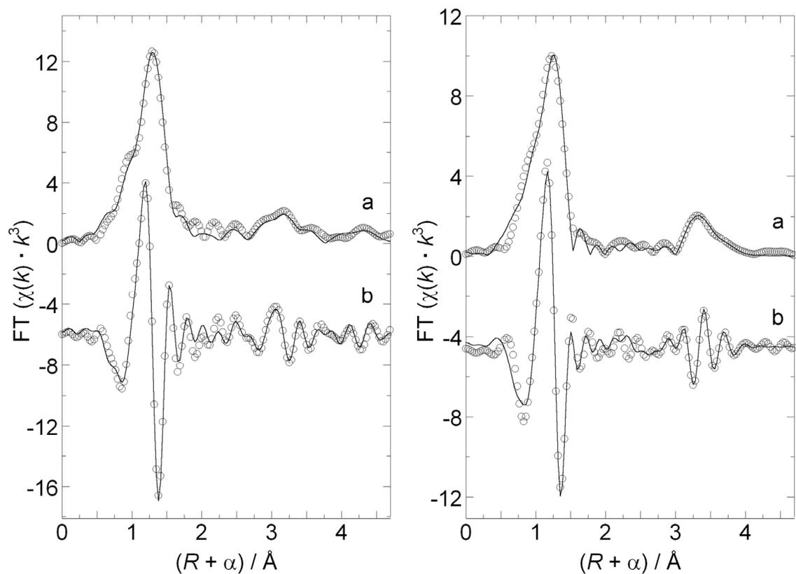
**Fig. S12.** Left: EXAFS (circles) and curvefit (line) for  $\text{MgMoO}_4$ , using a model that omits the Mo-Mg paths at 3.450 and 3.577  $\text{\AA}$ , as well as the Mo-Mg-O path at 3.770  $\text{\AA}$ . Right: EXAFS (circles) and curvefit (line) for  $\text{MgMo}_2\text{O}_7$ , using a model that omits the Mo-Mo-O path at 3.748  $\text{\AA}$ . The FT magnitude (a) and real component (b) are shown. Curvefit parameters can be found in Tables S3 and S4.
