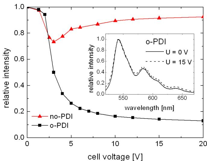
*Figure S3:* Relative fluorescence intensities of o-PDI (squares) and no-PDI (triangles) as a function of cell voltage. The inset shows the fluorescence intensity of o-PDI for two voltages. Excitation wavelength 488nm.
