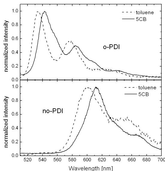
Figure S2: Normalized fluorescence spectra of PDI in toluene (broken line) and 5CB (full line) for o-PDI (top) and no-PDI (bottom) at excitation wavelength of 488 nm.
