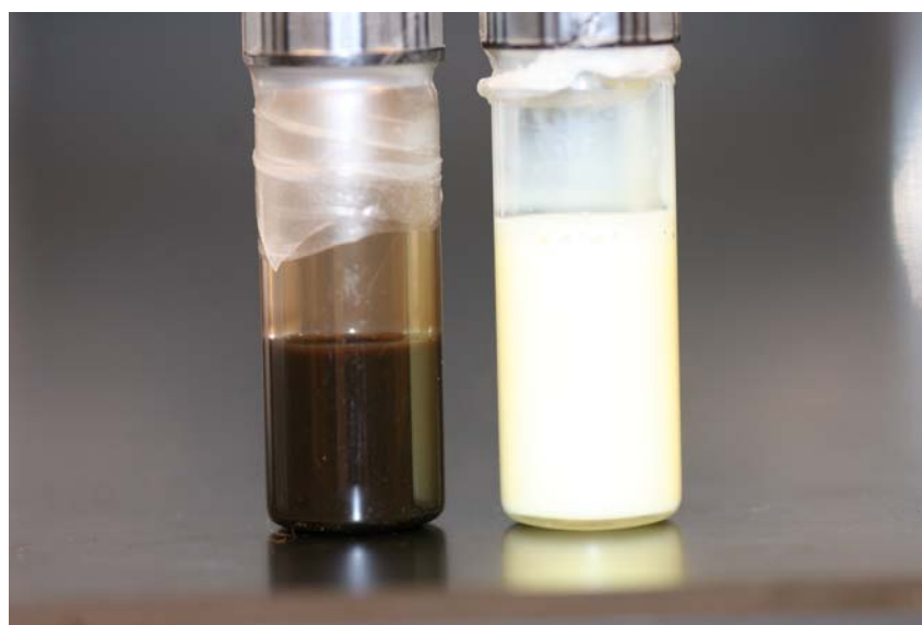
Figure S2. A typical image of two jetting solutions in vials where the dark one has p(AAm-co-AA) (5 wt/v %), PAA-stabilized magnetite (2.2 wt/v %), and rhodamine B isothiocyanate-dextran (0.5 wt/v %) in ethylene glycol, while the white solution has p(AAm-co-AA) (5 wt/v %), PAA-stabilized TiO 2 (2.2 wt/v %), and FITC-dextran (0.5 wt/v %) in ethylene glycol.
