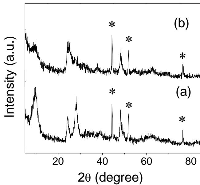
**Fig. S2** XRD patterns of (a) Na-TNT and (b) H-TNT. Symbols “\*” denote the internal standard Ni.
