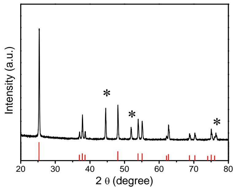
**Fig. S1** XRD pattern of the starting material of anatase  $\text{TiO}_2$ . Asterisks \* denote the internal standard Ni. The bottom bars denote the standard diffraction data of anatase  $\text{TiO}_2$  (JCPDS, No. 21-1272).
