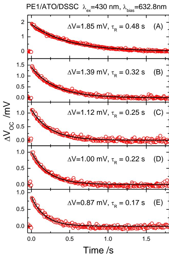
**Figure S7:** Photovoltage transients of PE1/ATO solar cells obtained at an open-circuit condition with pulse excitation at 430 nm under bias illumination at 632.8 nm for photon fluxes  $I_0/10^{15} \text{ cm}^{-2} \text{ s}^{-1} =$  (A) 2.2, (B) 4.7, (C) 6.3, (D) 7.3, and (E) 11. The transient data (circles) were fitted according to a simple kinetic model described in the text.
