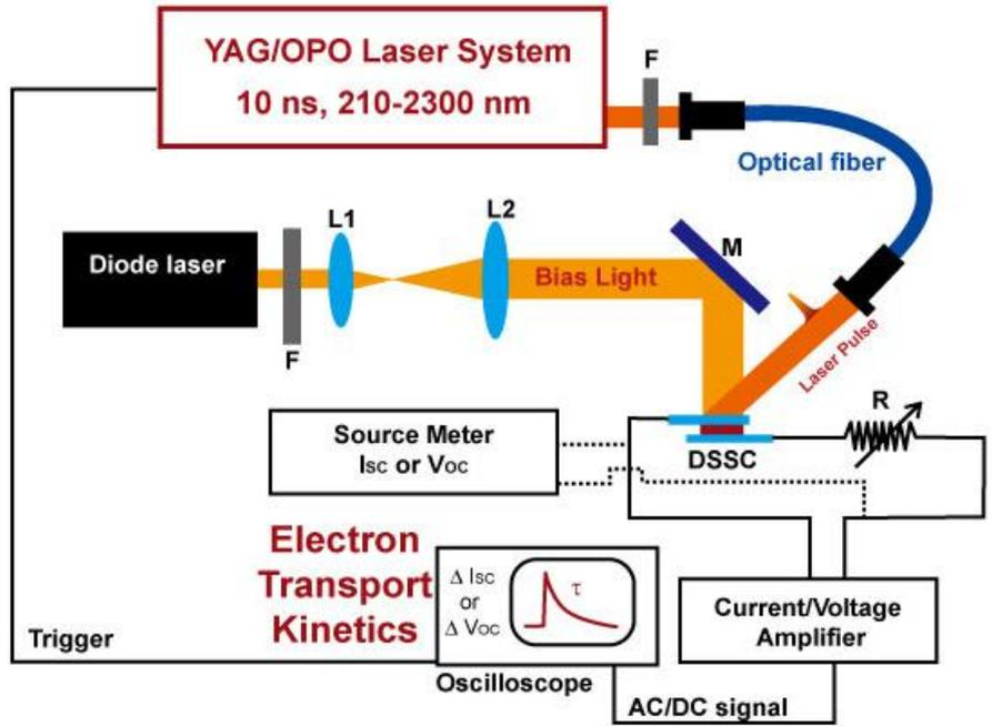
F: ND filter, L: lens, M: mirror, R: tunable resistance, DSSC: dye-sensitized solar cell
