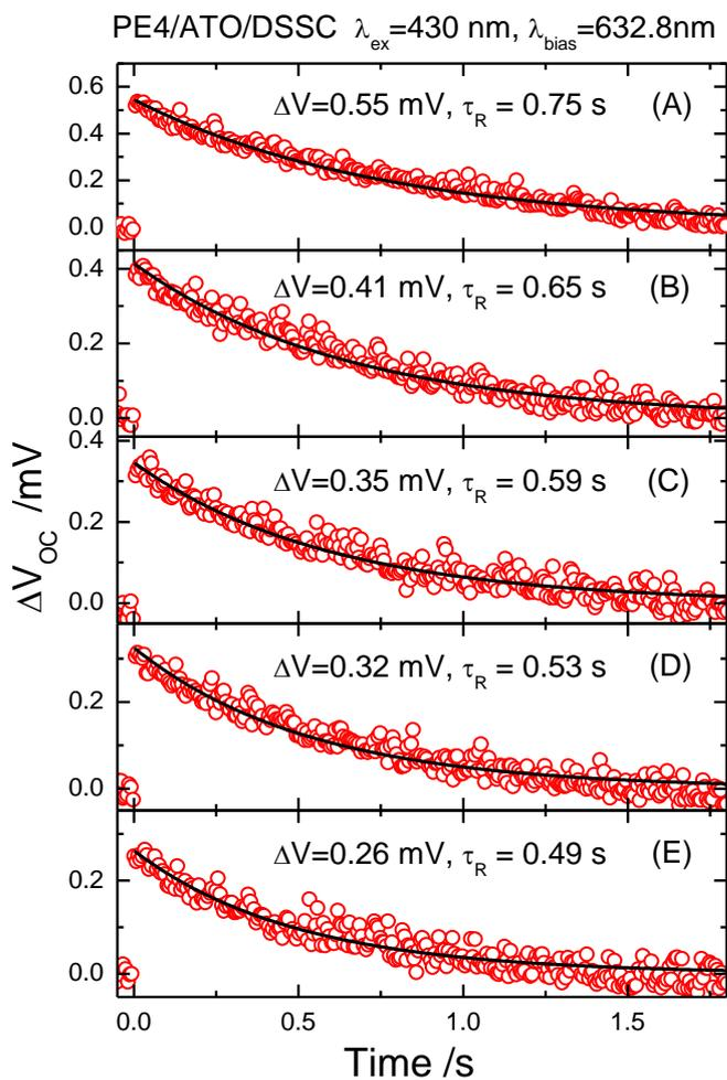
**Figure S10:** Photovoltage transients of PE4/ATO solar cells obtained at an open-circuit condition with pulse excitation at 430 nm under bias illumination at 632.8 nm for photon fluxes  $I_0/10^{15} \text{ cm}^{-2} \text{ s}^{-1} =$  (A) 2.2, (B) 4.7, (C) 6.3, (D) 7.3, and (E) 11. The transient data (circles) were fitted according to a simple kinetic model described in the text.
