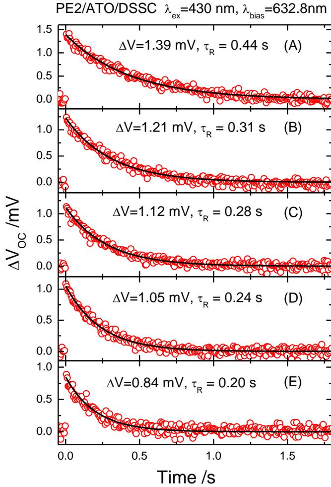
**Figure S8:** Photovoltage transients of PE2/ATO solar cells obtained at an open-circuit condition with pulse excitation at 430 nm under bias illumination at 632.8 nm for photon fluxes  $I_0/10^{15} \text{ cm}^{-2} \text{ s}^{-1} =$  (A) 2.2, (B) 4.7, (C) 6.3, (D) 7.3, and (E) 11. The transient data (circles) were fitted according to a simple kinetic model described in the text.
