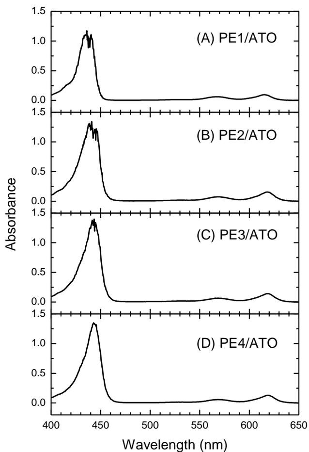
**Figure S1:** Absorption spectra of ATO NT films sensitized with (A) PE1, (B) PE2, (C) PE3 and (D) PE4. These sensitized films were fabricated into NT-DSSC devices for measurements of photovoltaic curves and photocurrent/photovoltage transients. The amounts of dye loading /nmol cm<sup>-2</sup> were determined to be 84, 90, 88 and 86 for PE1-PE4, respectively.
