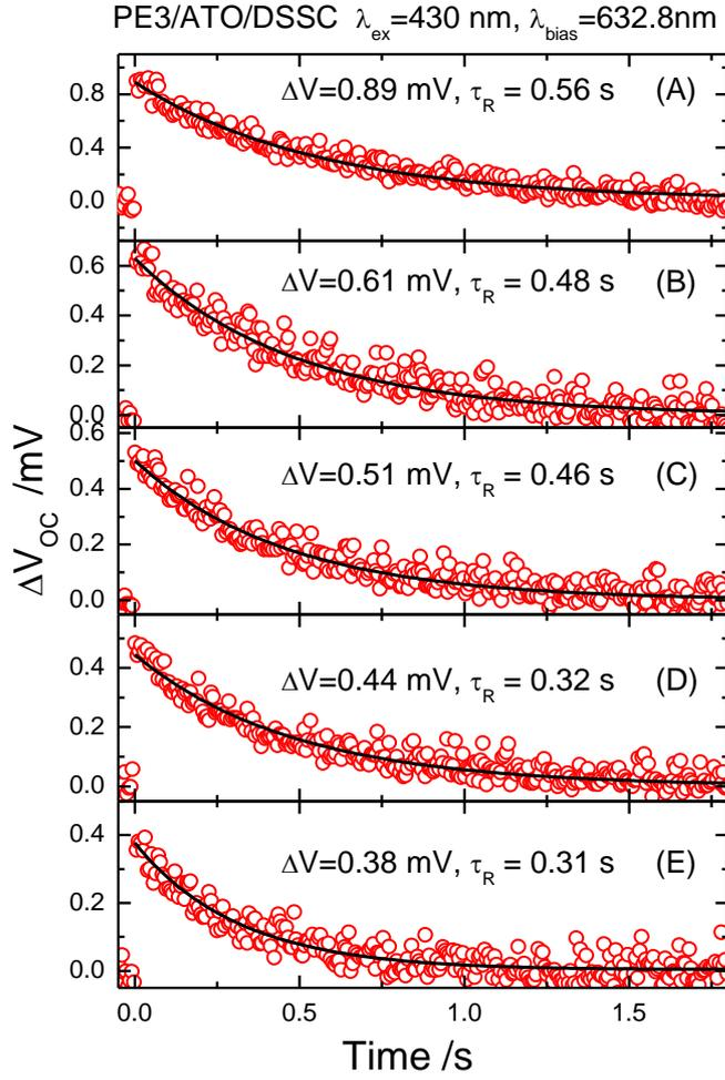
**Figure S9:** Photovoltage transients of PE3/ATO solar cells obtained at an open-circuit condition with pulse excitation at 430 nm under bias illumination at 632.8 nm for photon fluxes  $I_0/10^{15} \text{ cm}^{-2} \text{ s}^{-1} =$  (A) 2.2, (B) 4.7, (C) 6.3, (D) 7.3, and (E) 11. The transient data (circles) were fitted according to a simple kinetic model described in the text.
