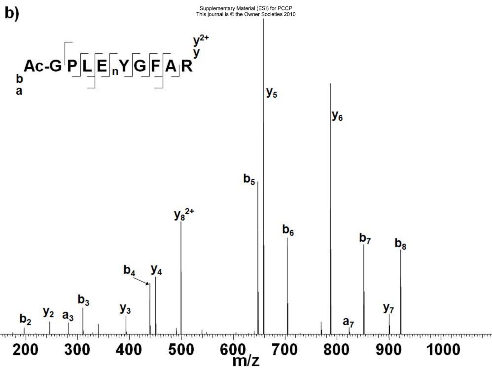
CID was completed on a Thermo Finnigan LTQ FT Ultra, with ions isolated and fragmented in the linear ion trap and transferred to the ICR cell for detection. AGC target was  $2 \times 10^5$ , maximum fill time 1 s. Isolation width was m/z 5. CID experiments were performed with helium gas at normalised collision energy 35 %. Each CID scan comprises four co-added microscans. Mass spectra shown comprise of 30 averaged scans.
