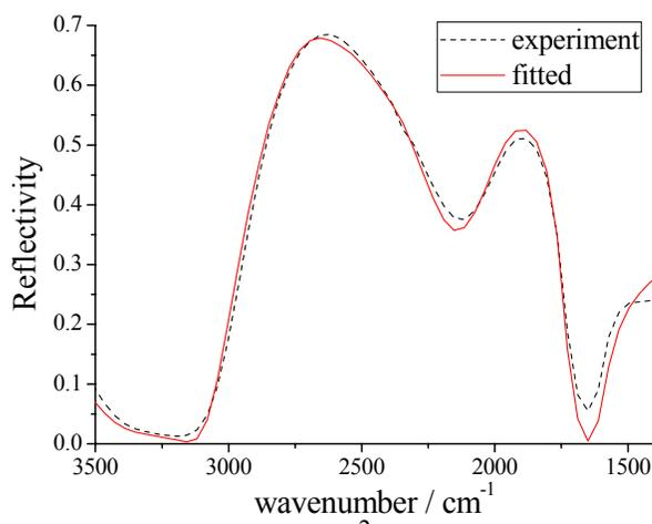
Fig. 2 Experimental (dashed line) and fitted IR reflectivity (dotted line) of the Pt(111) electrode in 0.1 M Na<sub>2</sub>SO<sub>4</sub> + 0.001 M H<sub>2</sub>SO<sub>4</sub> solution for p-polarized light. The fitted incident angle and water gap thickness are 28.5° and 5.0  $\mu\text{m}$
