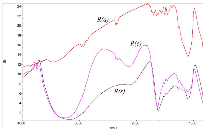
Fig. 1 Single beam reflectivities from:  $R(e)$  – Pt|H<sub>2</sub>O|ZnSe;  $R(a)$  – air|ZnSe and  $R(s)$  – H<sub>2</sub>O|ZnSe interface when the system was optimized to angle incidence  $\sim 31^\circ$ .
