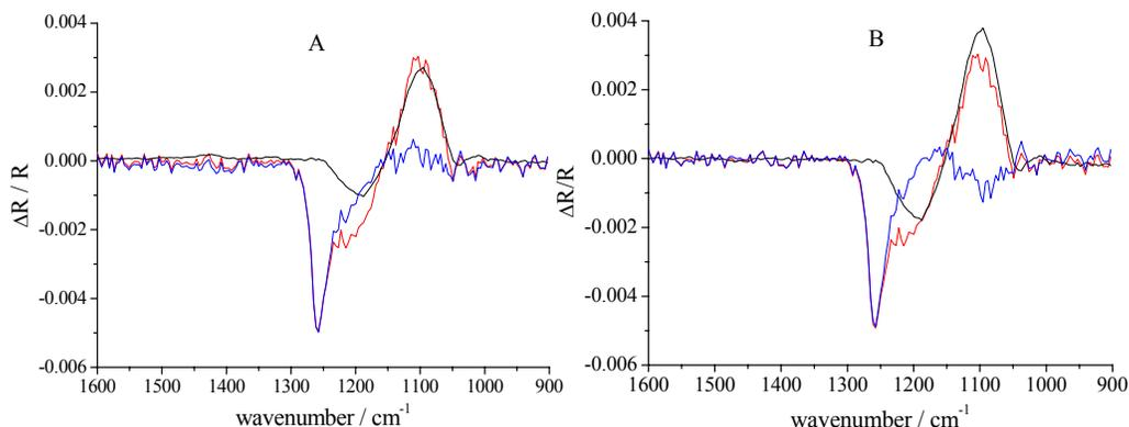
Fig. 7 Calculated IR spectra of the Pt(111) electrode in 0.1 M Na<sub>2</sub>SO<sub>4</sub> + 0.001 M H<sub>2</sub>SO<sub>4</sub> solution in terms of  $\left(\frac{\Delta R}{R}\right)_p$  (red),  $\left(\frac{\Delta R}{R}\right)_s \times \frac{\langle E_{p,ave} \rangle^2}{\langle E_{s,ave} \rangle^2}$  (black) and  $\left(\frac{\Delta R}{R}\right)_p - \left(\frac{\Delta R}{R}\right)_s \times \frac{\langle E_{p,ave} \rangle^2}{\langle E_{s,ave} \rangle^2}$  (blue).
