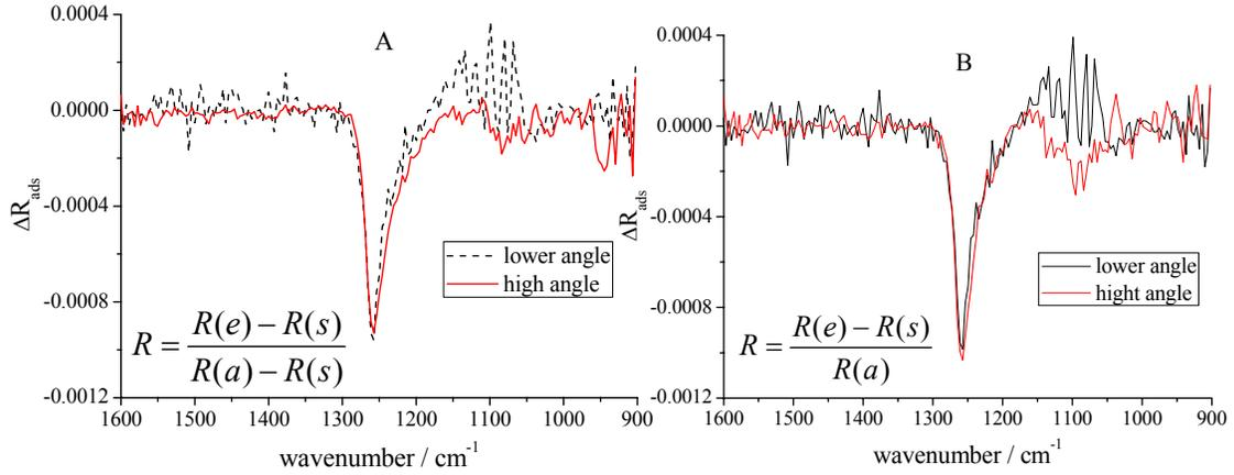
Fig. 11  $\Delta R_{ads}$  spectra calculated for the two experiments; red line  $31^\circ$  and black line  $28^\circ$  angle of incidence. The reflectivity of electrode surface is calculated by different formulas.
