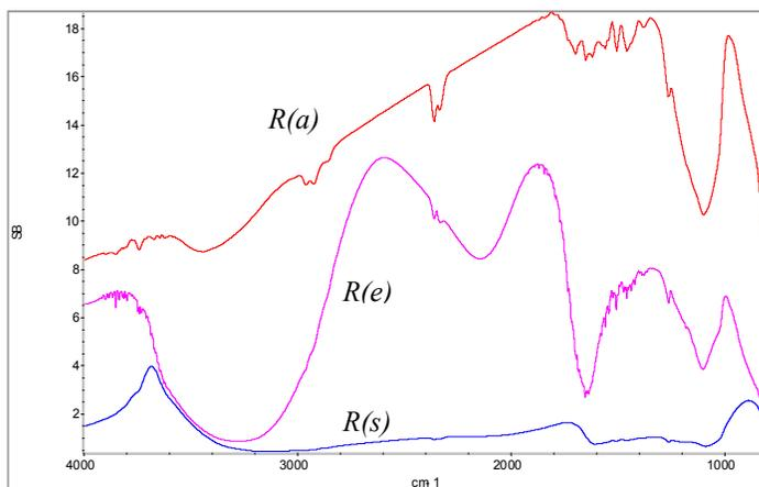
Fig. 8 Single beam reflectivities obtained from:  $R(e)$  – Pt|H<sub>2</sub>O|ZnSe;  $R(a)$  – air|ZnSe and  $R(s)$  – H<sub>2</sub>O|ZnSe interface when the system was optimized to angle incidence  $\sim 28^\circ$  in a 0.1 M Na<sub>2</sub>SO<sub>4</sub> + 0.001 M H<sub>2</sub>SO<sub>4</sub> solution.
