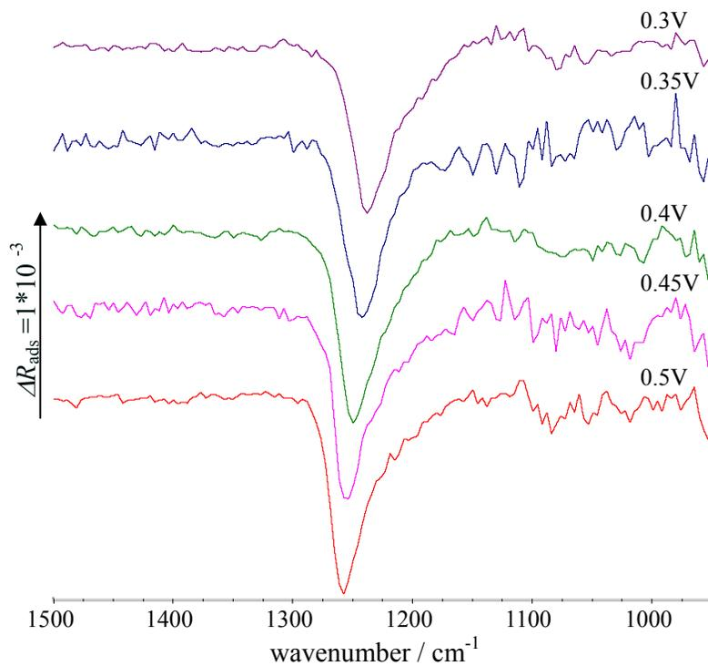
Fig. 14  $\Delta R_{ads}$  spectra of the Pt(111) electrode in 0.1 M  $\text{Na}_2\text{SO}_4$  + 0.001 M  $\text{H}_2\text{SO}_4$  solution.  $E_S$  is indicated in the figure.
