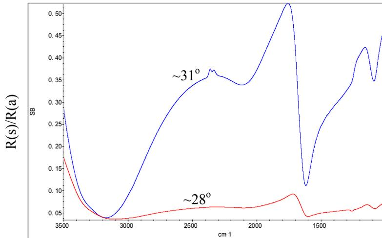
Fig. 4 Ratio of reflectivities from the window|solution to the window|air interface for two configurations of the experimental system optimized for the angle of incidence  $\sim 31^\circ$  and  $\sim 28^\circ$  (p-polarized light).
