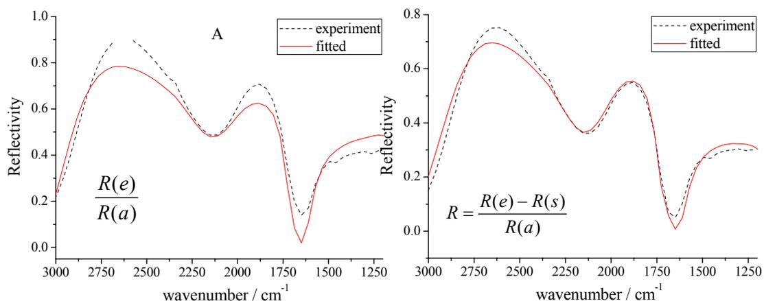
Fig. 9 Fits of the thin cavity thickness for the Pt(111) electrode in  $0.1 \text{ M Na}_2\text{SO}_4 + 0.001 \text{ M H}_2\text{SO}_4$  solution with the setup aligned for  $\sim 28^\circ$  angle of incidence. Left panel shows the fit for  $R(e)/R(a)$  and right panel is the fit for  $\{R(e)-R(s)\}/R(a)$ . The angle of incidence and thin cavity thickness for the right panel is  $28^\circ$  and  $4.1 \mu\text{m}$ , respectively.
