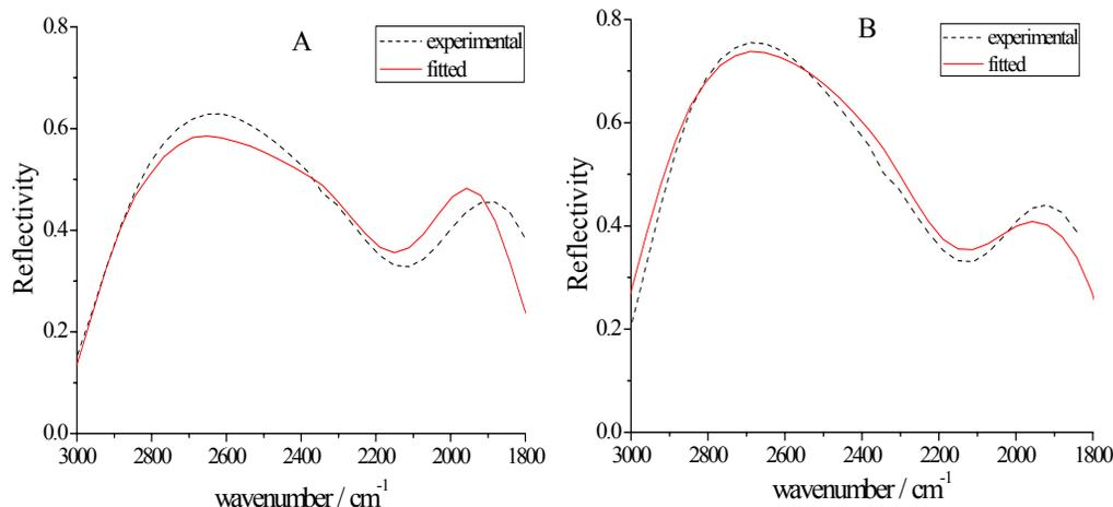
Fig. 6 Experimental and fitted IR reflectivity of the Pt(111) electrode in 0.1 M  $\text{Na}_2\text{SO}_4$  + 0.001 M  $\text{H}_2\text{SO}_4$  solution for p-polarized light. A: The fitted angle of incidence and cavity thickness are  $31^\circ$  and 4.9  $\mu\text{m}$ . B: The fitted angle of incidence and the cavity thickness are  $31^\circ$  and 2.8  $\mu\text{m}$ .
