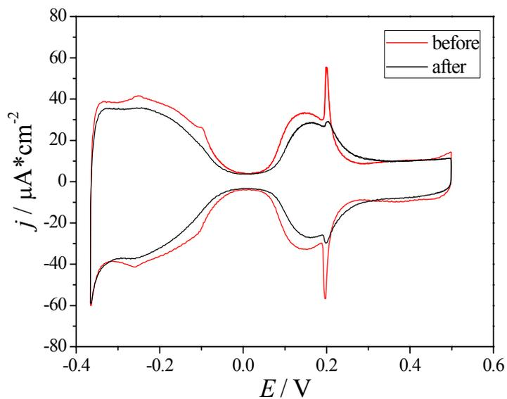
Fig. 12 CV curves of the Pt(111) electrode 0.001 M  $\text{H}_2\text{SO}_4$  + 0.1 M  $\text{Na}_2\text{SO}_4$  solution before and after IR experiment. The scan rate is  $50 \text{ mV}\cdot\text{s}^{-1}$
