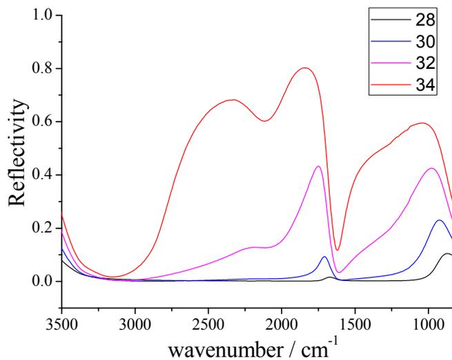
Fig. 5 For ZnSe|H<sub>2</sub>O system, simulated  $R(s)/R(a)$  curves for various angles of incidence, p-polarized light.
