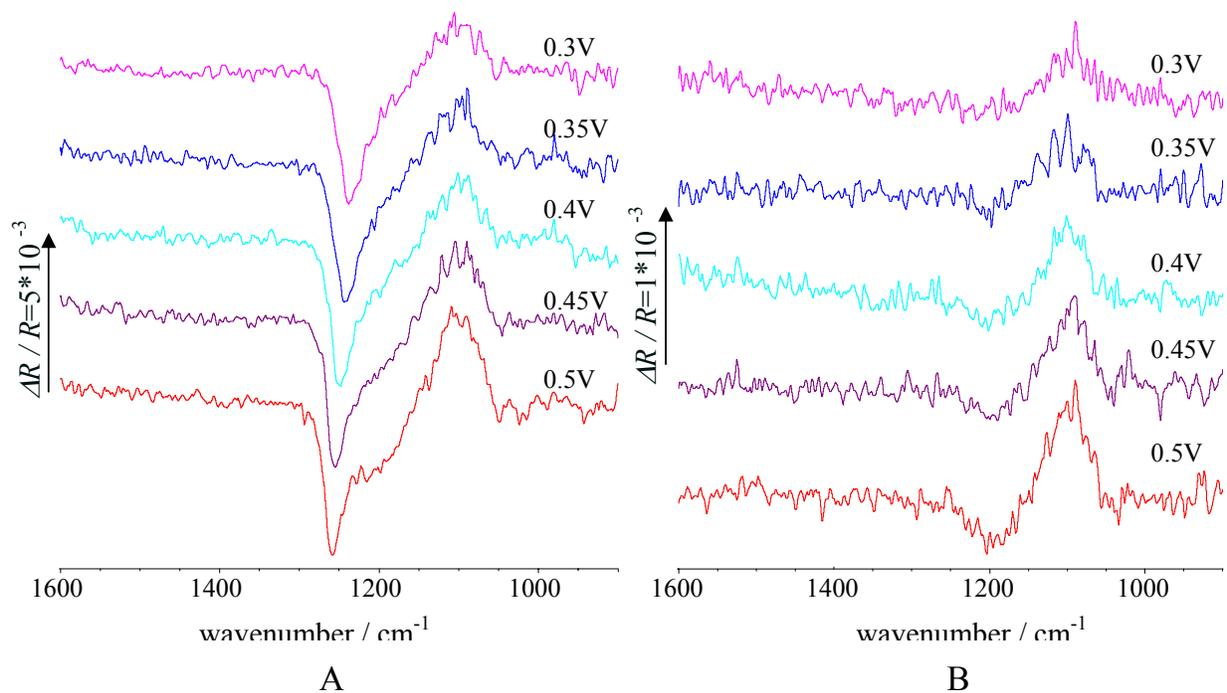
Fig. 13 SNIFTIRS spectra of the Pt(111) electrode in 0.1 M Na<sub>2</sub>SO<sub>4</sub> + 0.001 M H<sub>2</sub>SO<sub>4</sub> solution at (A) p-polarized light, and (B) s-polarized light.  $E_S$  is indicated in the figure, and  $E_R$  is 0.04 V.
