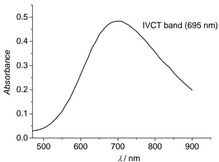
**Fig. A.** UV-Vis absorption spectrum of PB nanoparticles in solution.
