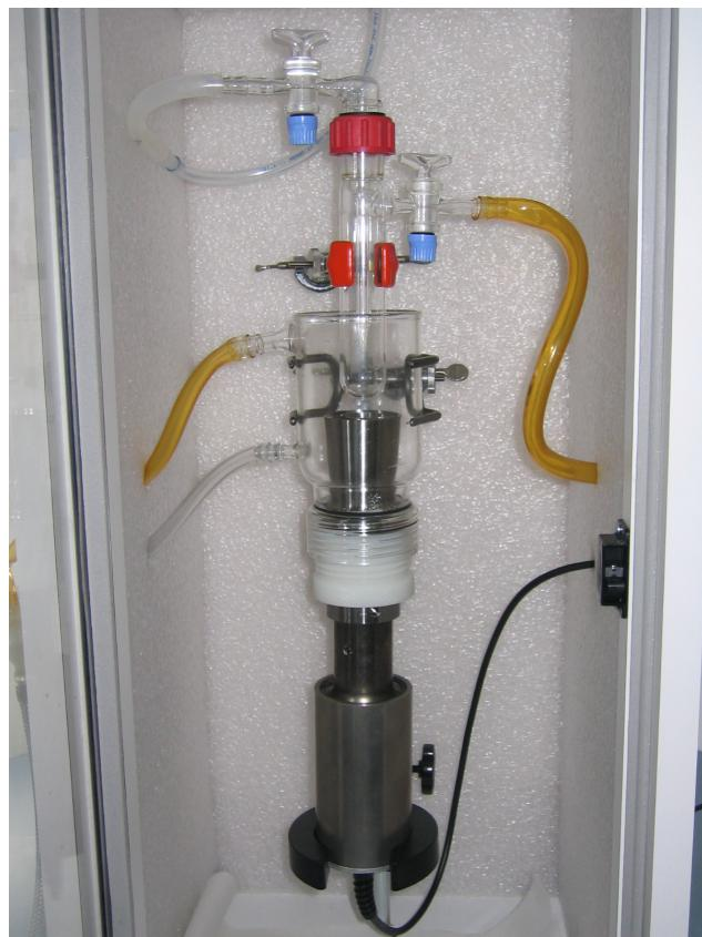
**Figure 1S.** Cup-horn sonochemical reactor without direct contact of sonicated liquid with ultrasonic emitter.
